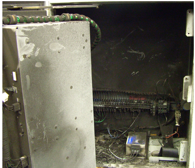
Fig. 3. Burned-Out Recloser Control
