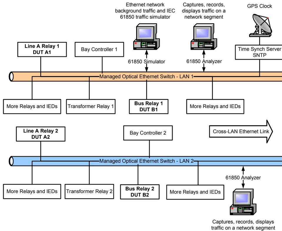
(b) Full interconnection of LAN devices simulating field application
