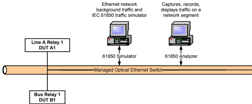
(a) Equivalent test in which DUT interacts with simulator for the rest of the LAN devices
