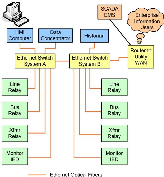
Fig. 2. Typical Substation-Bus LAN Implementation
