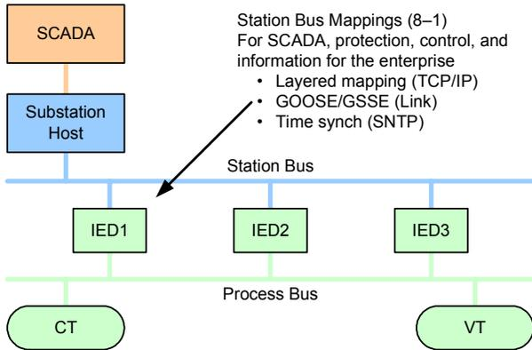
Fig. 1. IEC 61850 Station Bus and Process Bus Levels
