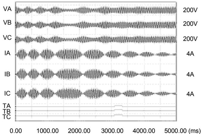
Fig. 7 Misoperation when the power system recovers from a swing
