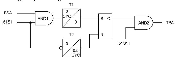
Fig. 9 Single-pole trip logic for high-impedance ground faults
