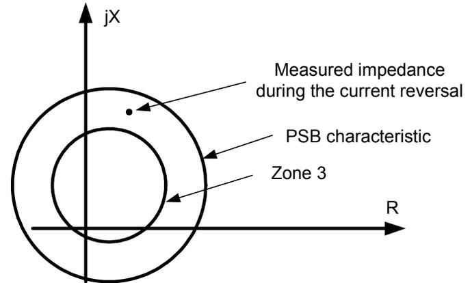
Fig. 4 The location of measurement impedance
