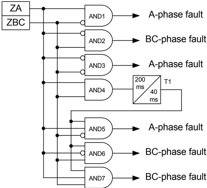
Fig. 6 Logic diagram for faulted phase selection during power swings
