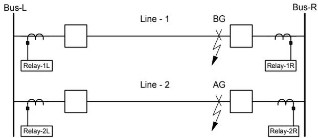
Fig. 10. Evolving fault on a double-circuit system
