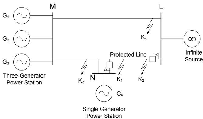
Fig. 2 Short three-terminal ring network
