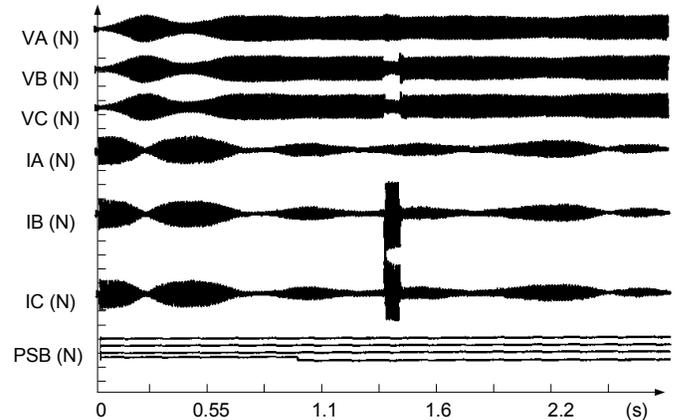
Fig. 8 A loss-of-potential problem caused failed operation for a fault
