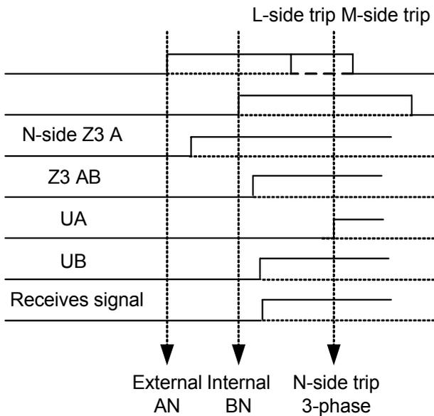
Fig. 5 Sequence of protection elements in Example II
