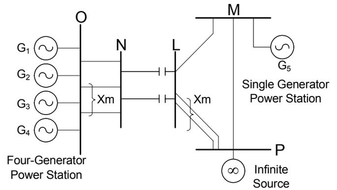
Fig. 3 The system with series compensation
