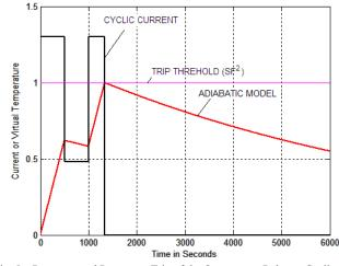
Fig. 5 Response and Premature Trip of the Overcurrent Relay to Cyclic Overload.
