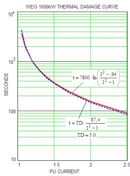
Fig. 3 Thermal Damage Curve with Thermal Model and a Coordinated Motor Relay Characteristic
