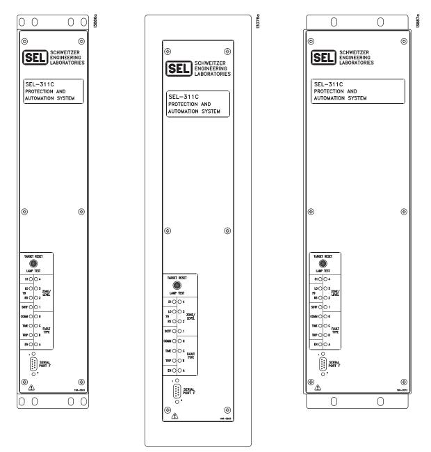
Figure 17 SEL-311C Vertical Front-Panel Diagrams
