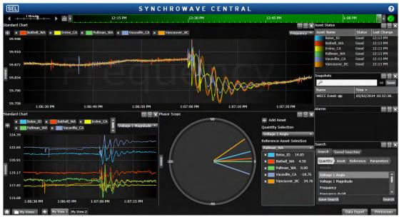
Figure 9 SYNCHROWAVE Central Real-Time Wide-Area Visualization Tool
