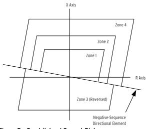
Figure 5 Quadrilateral Ground-Distance Characteristics
