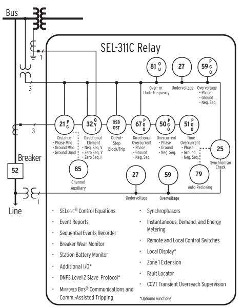
Figure 1 Functional Diagram
