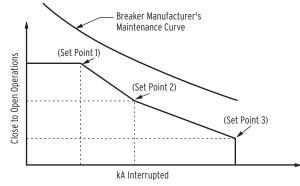
Figure 10 Breaker Contact Wear Curve and Settings
