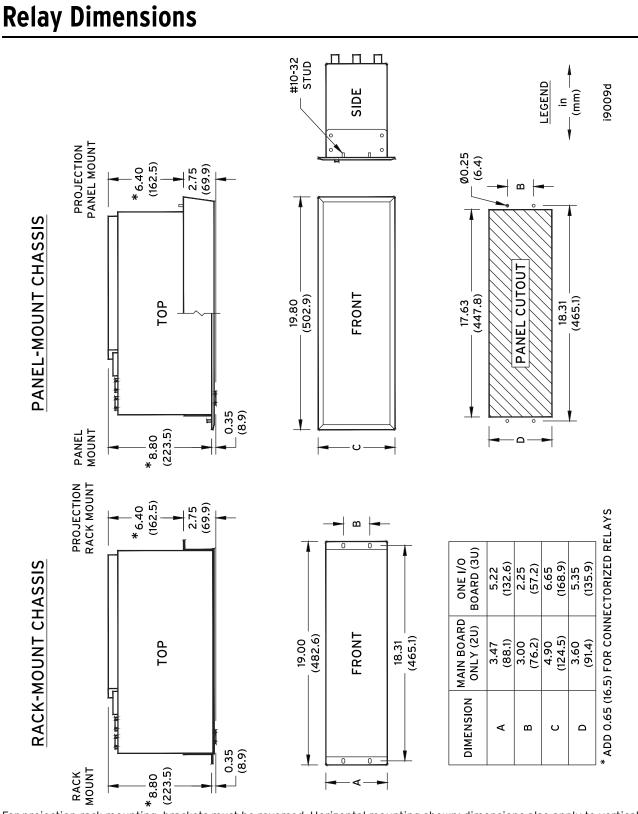
For projection rack mounting, brackets must be reversed. Horizontal mounting shown; dimensions also apply to vertical mounting.
