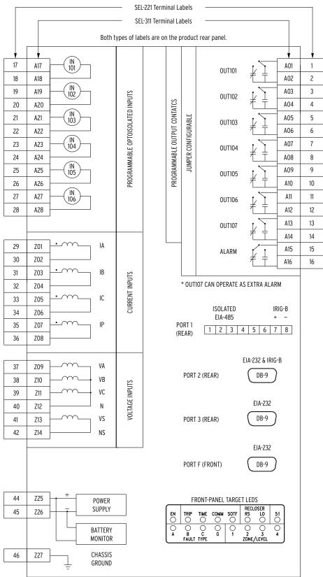
Figure 15 SEL-311C Inputs, Outputs, and Communications Ports
