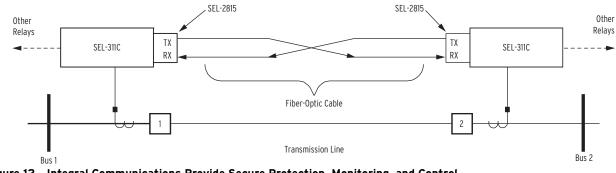
Figure 12 Integral Communications Provide Secure Protection, Monitoring, and Control
