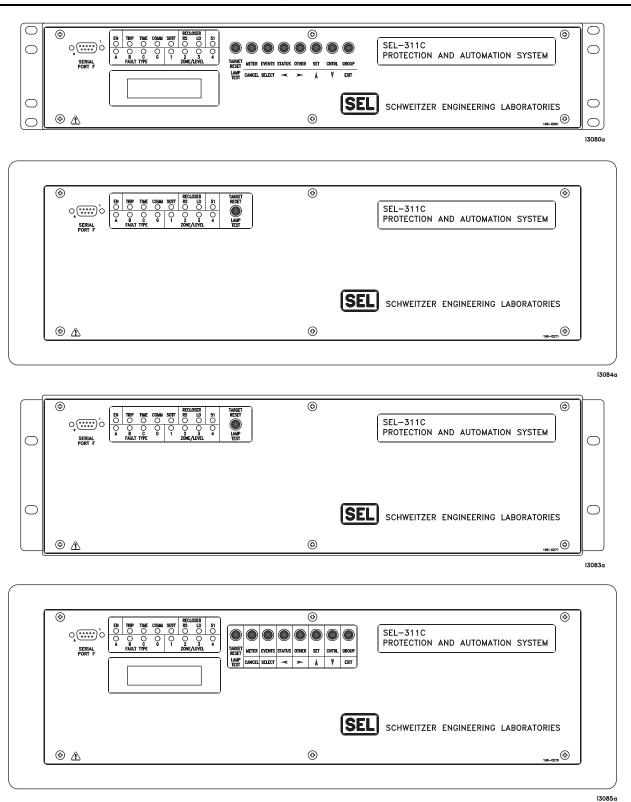
Figure 16 SEL-311C Horizontal Front-Panel Diagrams
