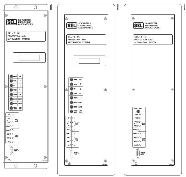
Figure 18 More SEL-311C Vertical Front-Panel Diagrams
