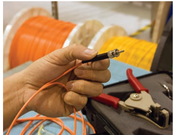
Finished! A connectorized cable is ready to plug in to your application.
