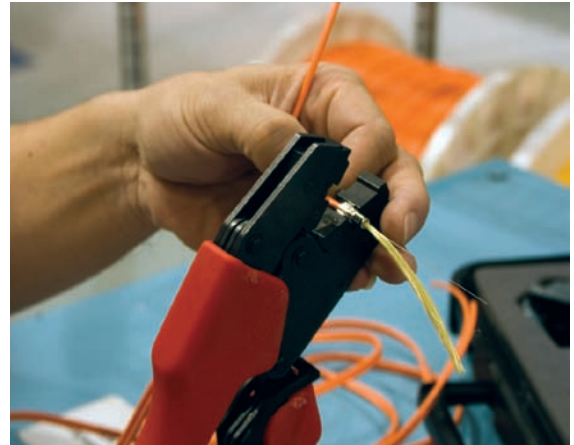
Crimp the connector directly onto the outer jacket for strong, solid connector retention.
