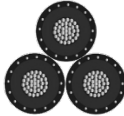
Single-Phase Triplexed XLPE With Nonmagnetic Concentric Neutral or Foil Tape
