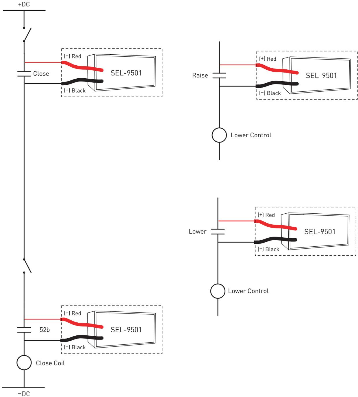
Typical SEL-9501 Contact Arc Suppressor Application
