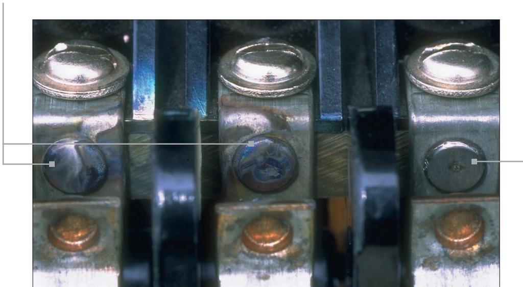
The unprotected contacts show burning, pitting, and discolorization, while the contact protected by the SEL-9501 remains undamaged.
