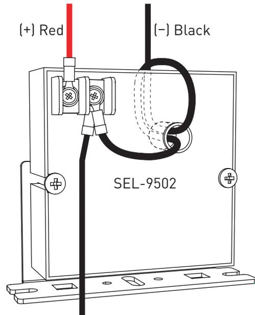
To apply the SEL-9502 to circuits with load current less than 1 A, wrap the negative terminal lead through the hole in the SEL-9502 twice, as shown. Placing two turns through the current sense circuit of the SEL-9502 allows it to reliably sense currents as low as 0.4 A.
