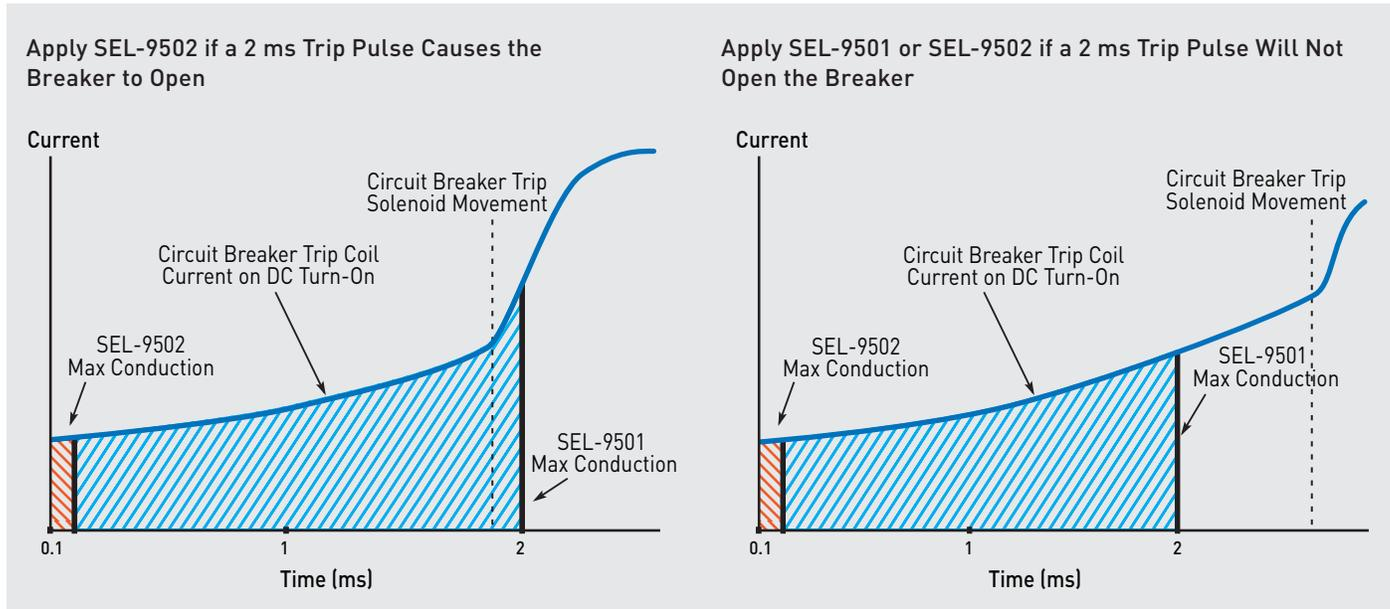
These graphs show a circuit breaker's trip point compared to the current let-through time on dc turn-on for the SEL-9501 and SEL-9502. The SEL-9502 prevents unintentional trips by providing minimal current let-through.
