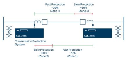
With step-distance protection, relays provide fast protection in Zone 1 and slow protection (20-40 cycle operation) in Zone 2.
