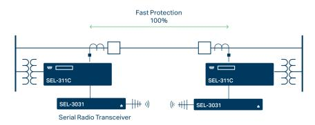
SEL-3031 radios enable fast protection (2-4 cycle operation) over 100 percent of the line. The scheme falls back to step-distance protection if communications fail.
