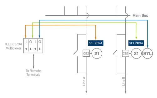
Fiber-optic communications isolate devices from ground-potential rise, EMI, and radio frequency interference (RFI).
