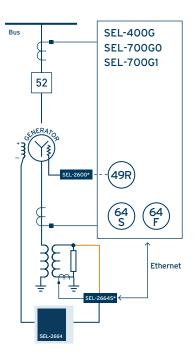
The SEL-2664 Field Ground Module can be directly connected to the SEL-300G Generator Relay, SEL-400G Advanced Generator Protection System, and versions of the SEL-700G Generator Protection Relay (i.e., SEL-700G0, SEL-700G1, SEL-700GT, and SEL-700GW) via a fiber-optic serial connection. The SEL-2664 may be connected to the SEL-2664S first and then to the SEL-400G, SEL-700G0, or SEL-700G1.
