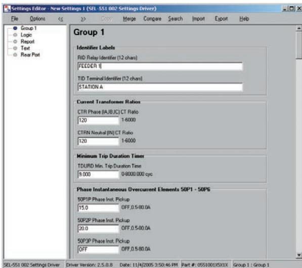
Develop settings using acSELERATOR® QuickSet™ SEL-5030 Software.
