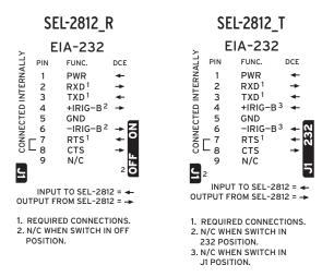
Figure 21 SEL-2812\_R and SEL-2812\_T Signal Flow
