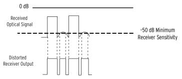
Figure 6 Effect of Reflections on Received Data
