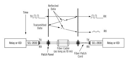
Figure 5 Data Reflected in Fiber-Optic Cables
