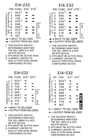
Figure 23 SEL-2815, SEL-2829, SEL-2830, and SEL-2831 Signal Flow
