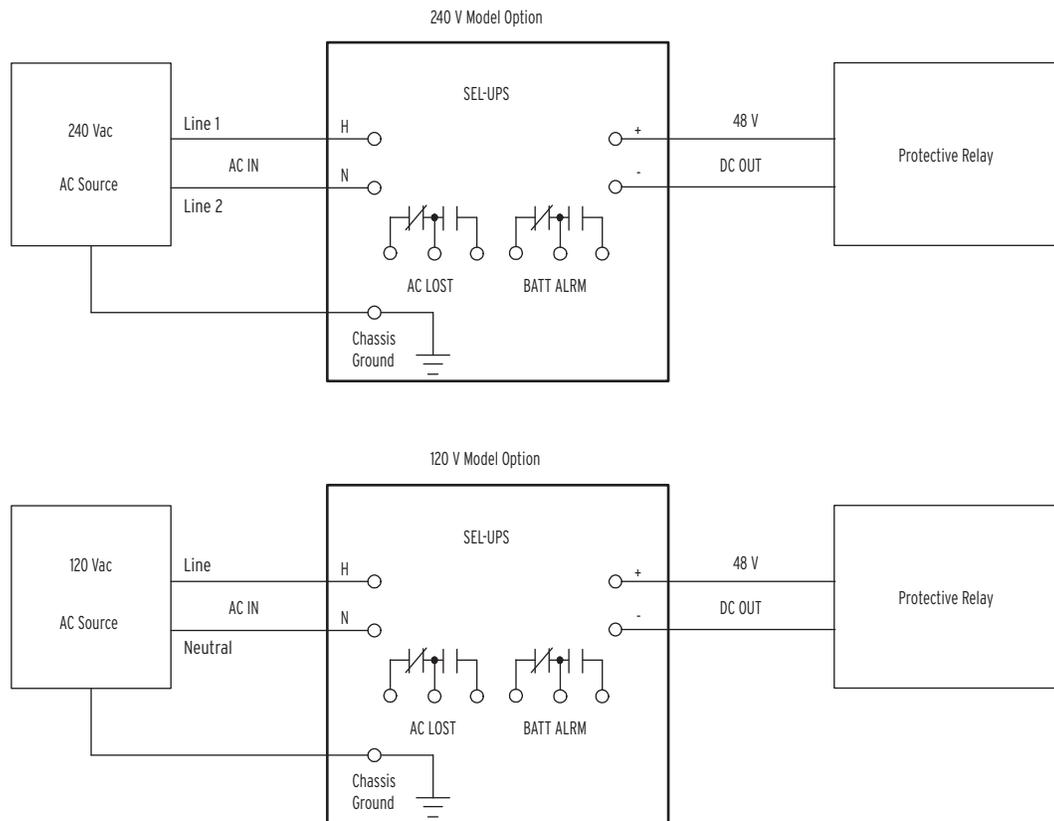
**Figure 1 Application Diagram**
