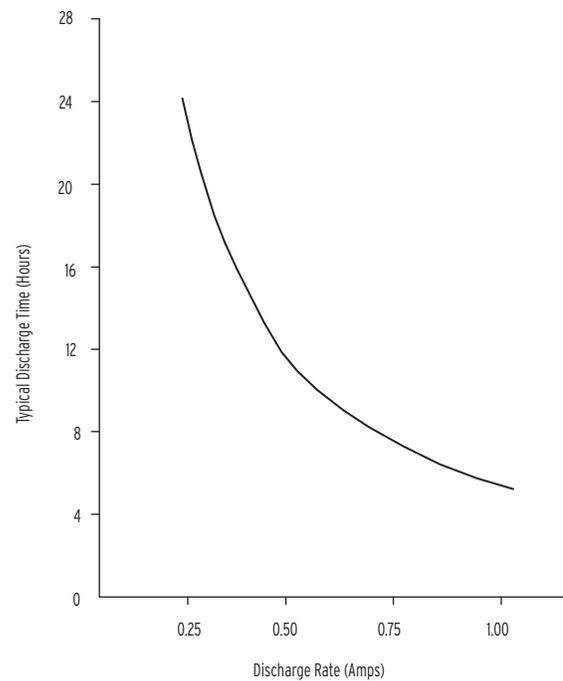
**Figure 3 Typical Discharge Time Versus Discharge Rate at +25°C**
