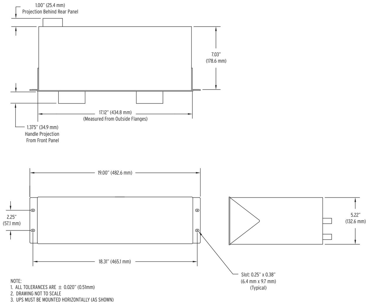
**Figure 4 SEL-UPS Dimensions, Panel Cutout, and Drill Plan**
