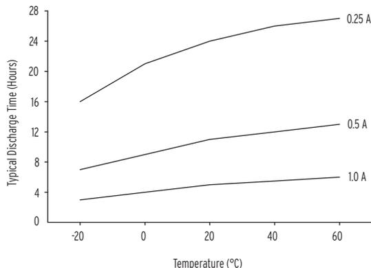
**Figure 2 Typical Discharge Time Versus Temperature at Various Discharge Rates**
