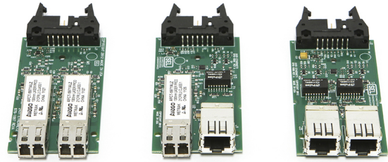
Figure 14 Ethernet Communications Cards
