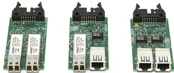
Figure 13 Ethernet Communications Cards
