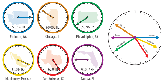
Figure 6 View of System Angle at Multiple Locations
