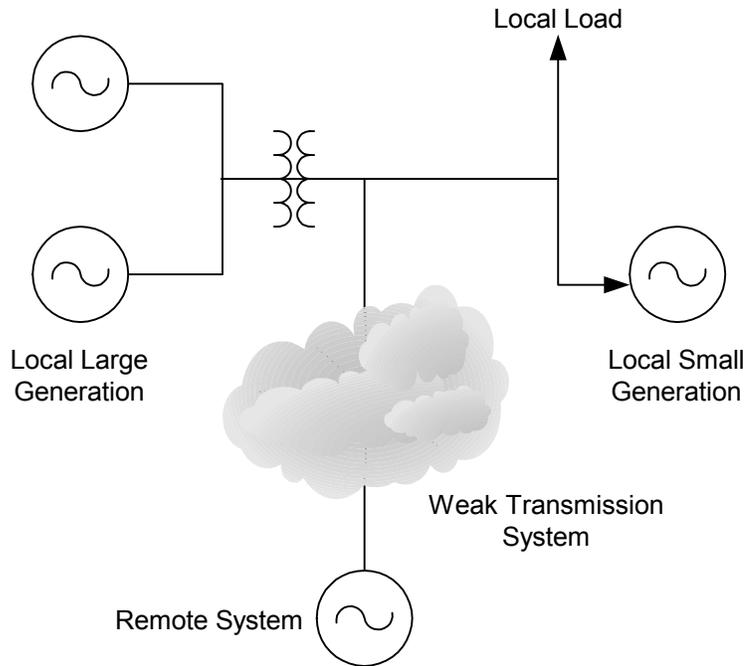
**Figure 6** Power System With Weak Transmission System
