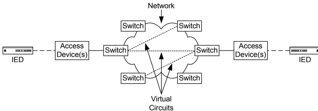
**Figure 4** Virtual Circuit on a Digital Communications Network
