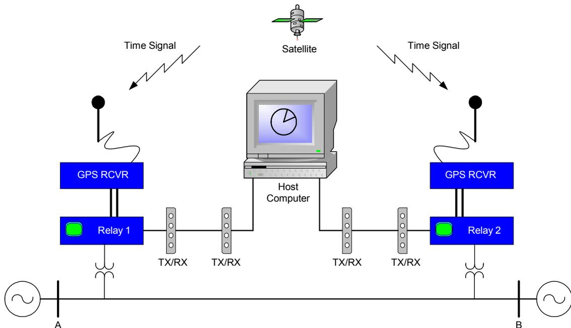
**Figure 3** Example Synchrophasor Monitoring System
