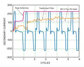
Figure 1—Engineers at SEL developed a patented filter technology that SEL calls Adaptive Overcurrent Element filtering. Combining the dc offset and harmonic immunity of the cosine filter, and the accurate magnitude acquisition of the peak filter, SEL's Adaptive Overcurrent Element provides "the winning combination" of both filters working at any given time.
