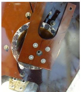
Figure 3—Inspection of the utility transformer revealed the damage caused to the rotor assembly (shown above) and the rotor of the tap changer (shown below) caused by arcing.
