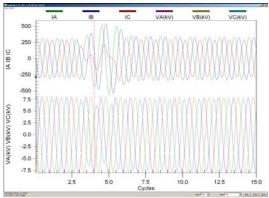
Figure 1—The customer detected a voltage problem and reviewed the SEL event report records using ACSELERATOR<sup>®</sup> Analytic Assistant SEL-5601 Software. The associated oscillograph (above) shows a problem with the three-phase voltage and current.
