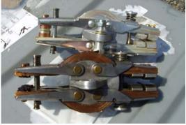
Figure 4—The old bridge contact is shown in the lower portion of this on-site photo. The contacts at both ends are severely worn. The new bridge contact at the top of the photo clearly shows what the contacts should look like.
