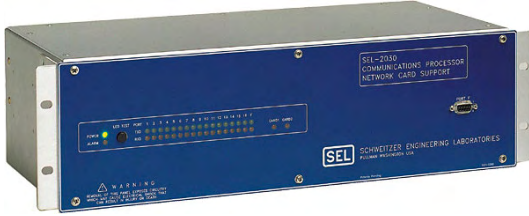
Figure 8—The SEL-2030 Communicators Processor provides quick and economic integration of Intelligent Electronic Devices (IEDs) into SCADA, local human-machine interface (HMI), and overall substation integration applications.
