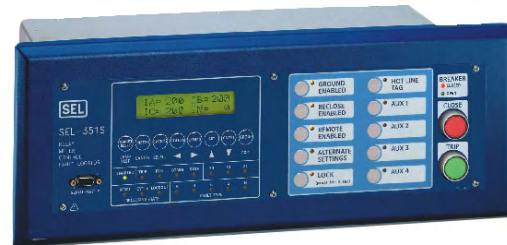
Figure 7—The SEL-351S includes a programmable four-shot auto-reclosing function with synchronism- and voltage-check logic to match a variety of reclosing practices.
