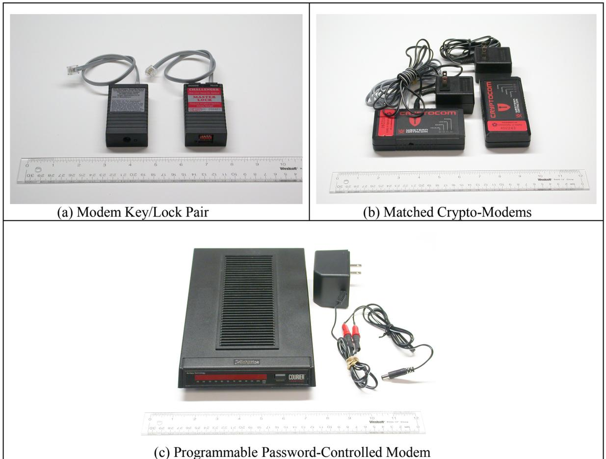
**Figure 5** Low-Cost Secure Modem Devices
