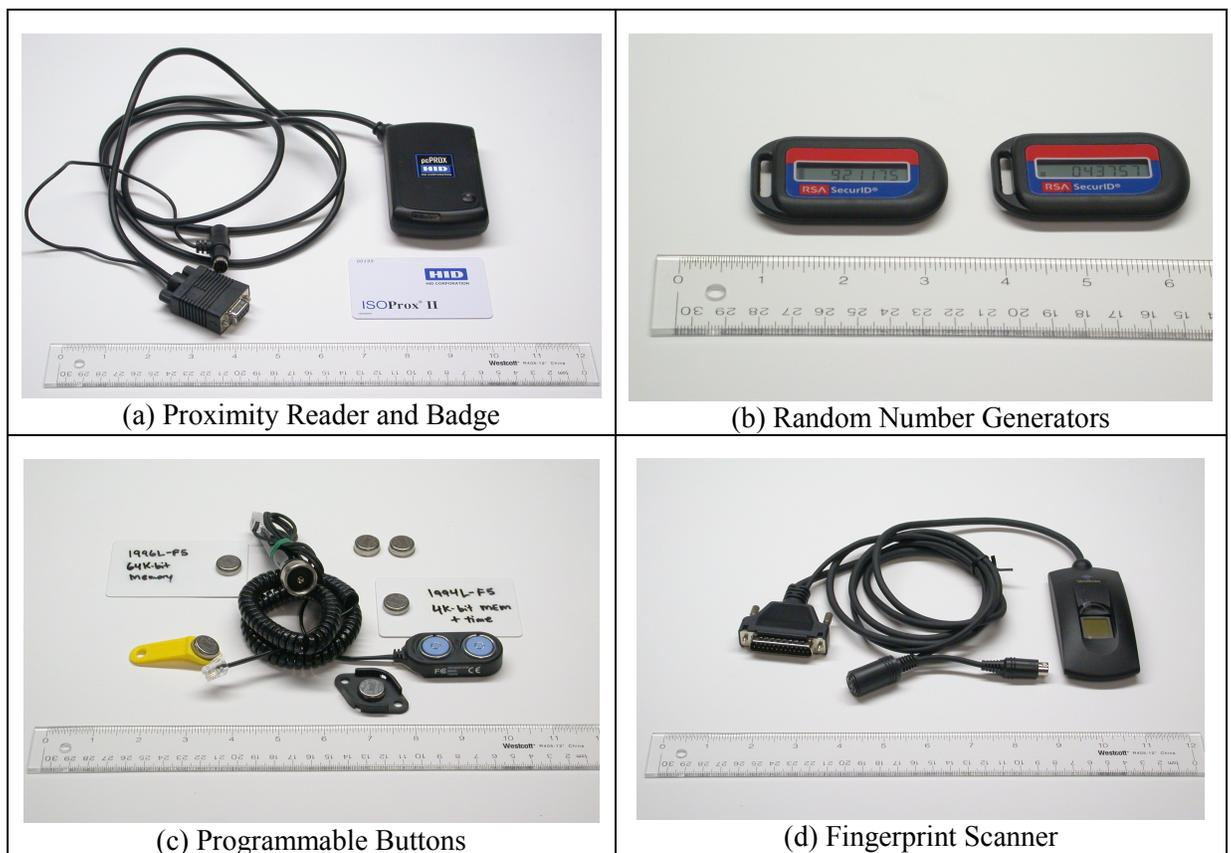
**Figure 2** Low Cost Authentication Devices
