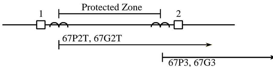
Figure 5: Basic DCB Scheme Protection
