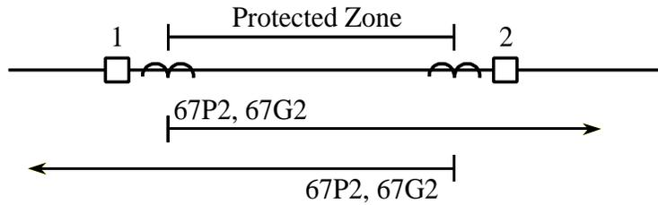
Figure 3: Basic POTT Scheme Protection
