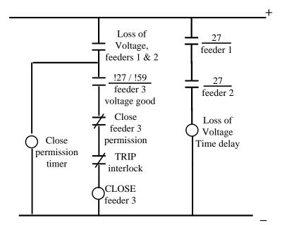
Figure 14: Control circuit representation of Automatic Source Transfer logic.
