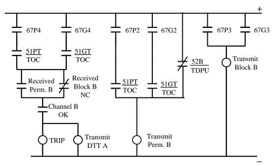
Figure 8: Control circuit representation of Overreaching POTT/DCB Scheme
