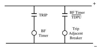
Figure 9: Control circuit representation of Breaker Failure Scheme
