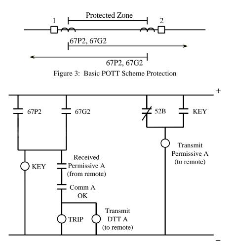
Figure 4: Control circuit representation of POTT logic
