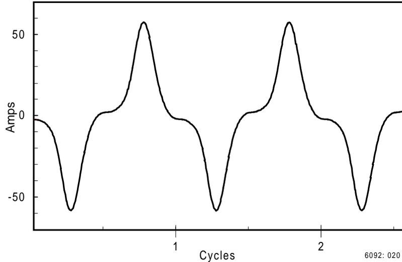
**Figure 21: Exciting Current During 150% Transformer Overvoltage Condition.**
