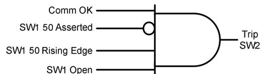
Fig. 30. Logic for Tripping SW2 for Fast Restoration of Line 2 Load Using Communications-Enhanced Scheme
