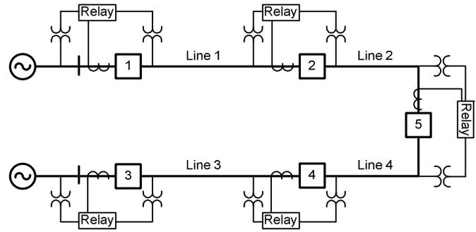
Fig. 20. One-Line Diagram of Conventional Restoration Scheme Using Relays and Voltage Transformers
