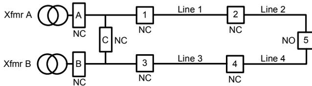
Fig. 4. System Single-Line Diagram (Two Source Transformers)
