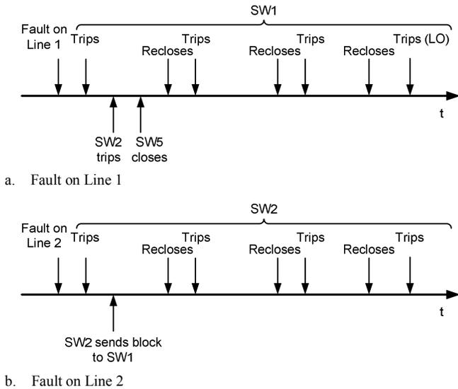
Fig. 33. Timing for Permanent Faults – Communications-Enhanced Scheme.
