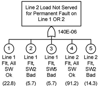
b. Unavailability of Serving Line 2 Load – Manual Isolation Switches
