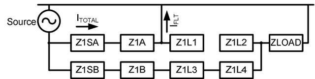
Fig. 7. Faulted System Sequence Connection Diagram (Independent Source Feed Example)
