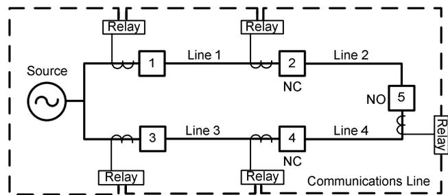
Fig. 26. One-Line Diagram of Communication-Enhanced Restoration Scheme
