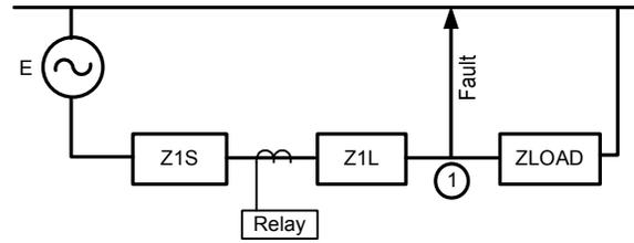
Secondary Values:  $E = 66.4 \text{ V } \angle 0^\circ$   $Z_{1S} = 1 \Omega \angle 90^\circ$   $Z_{1L} = 8 \Omega \angle 60^\circ$
