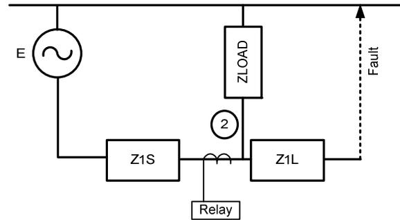
Secondary Values:  $E = 66.4 \text{ V } \angle 0^\circ$   $Z_{1S} = 1 \Omega \angle 90^\circ$   $Z_{1L} = 8 \Omega \angle 60^\circ$
