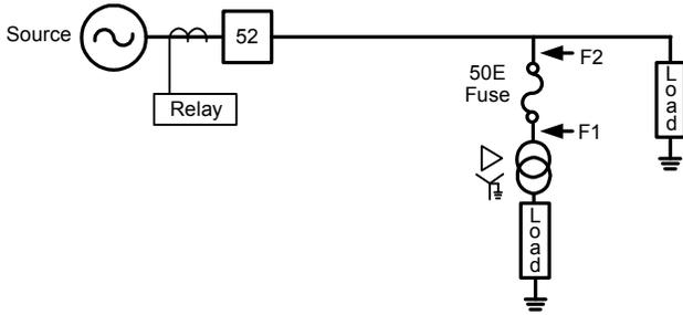
Fig. 15. System Single-Line Diagram for Evolving Fault Case Studies
