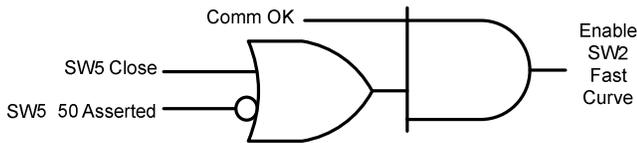
Fig. 32. SW2 Fast Curve Tripping Logic – Communications-Enhanced Scheme
