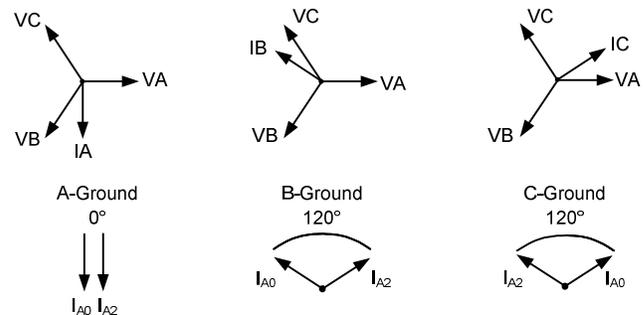
Fig. 16. Angle Relationship of  $I_{A2}$  and  $I_0$  for Single-Line-to-Ground Faults
