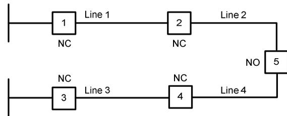
Fig. 19. One-Line Diagram With SW1 – SW4 Normally Closed, and SW5 Normally Open
