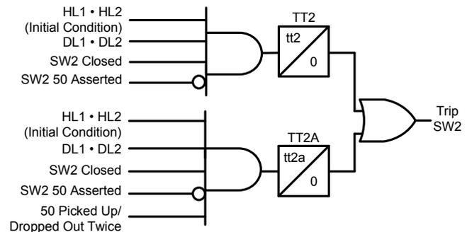
Fig. 21. Tripping Logic for SW2 – Conventional Restoration Scheme
