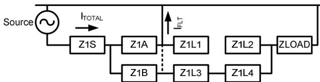
Fig. 5. Sequence Connection Diagram (Two Source Transformers)
