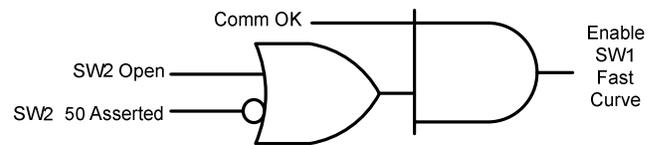
Fig. 29. SW1 Fast Curve Tripping Logic – Communications-Enhanced Scheme
