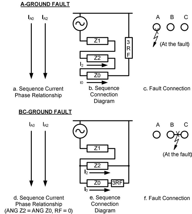
Fig. 17. Angle Relationship of  $I_{A2}$  and  $I_0$  for A-Ground and BC-Ground Faults
