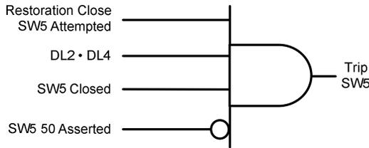
Fig. 23. Tripping Logic for Switch SW5 – Conventional Restoration Scheme
