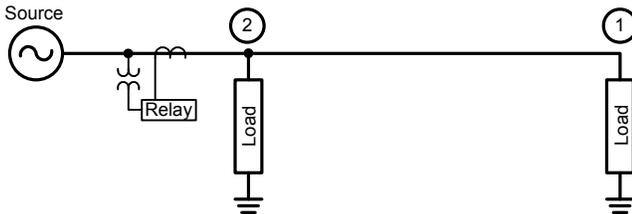
Secondary Values:  $E = 66.4 \text{ V } \angle 0^\circ$   $Z_{1S} = 1 \Omega \angle 90^\circ$   $Z_{1L} = 8 \Omega \angle 60^\circ$
