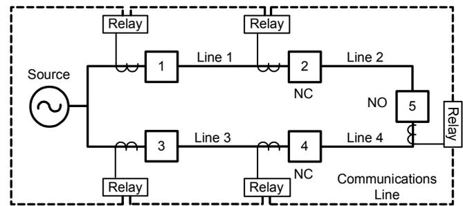
a. System Single-Line Diagram – Automatic Isolation Switches
