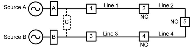
Fig. 6. System Single-Line Diagram (Independent Source Feed Example)
