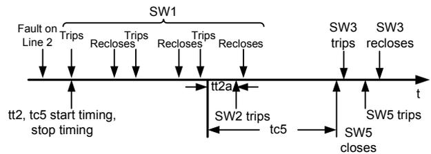
Fig. 25. Line 2 Permanent Fault Timing – Conventional Restoration Scheme
