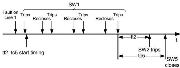
Fig. 24. Line 1 Permanent Fault Timing – Conventional Restoration Scheme
