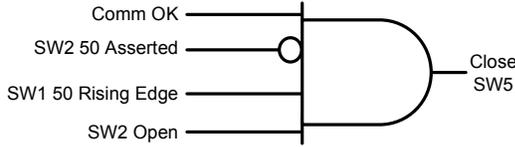
Fig. 31. Logic for Closing SW5 for Fast Restoration for Line Load Using Communications-Enhanced Scheme
