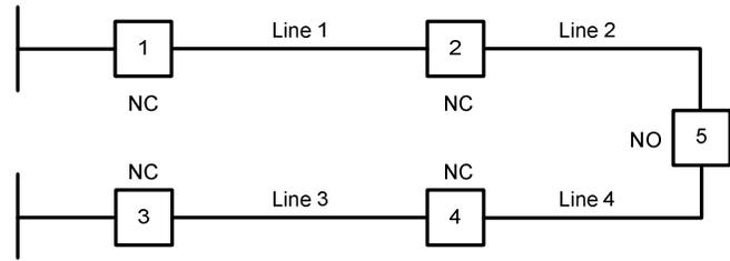
Fig. 28. One-Line Diagram With Switches 1 Through 4 Closed and Switch 5 Open
