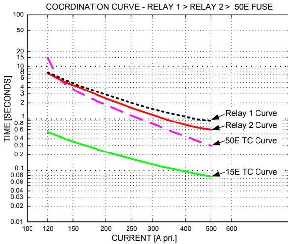
Fig. 9. Time Coordination Can Aggravate Power Quality for Line 1 Faults
