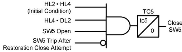
Fig. 22. Closing Logic for Switch SW5 – Conventional Restoration Scheme
