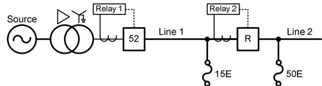
Fig. 8. System Single-Line Diagram of an Application Where Communications Improve Time Coordination
