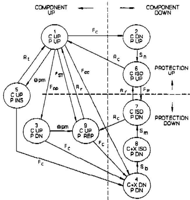
**Figure A.1: Markov Model of a Protection/Component System, Relay Includes Self-Tests**
