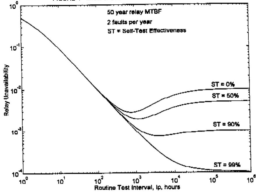
FIGURE 5 - Effect of Relay Self-Tests on Power System Unavailability
