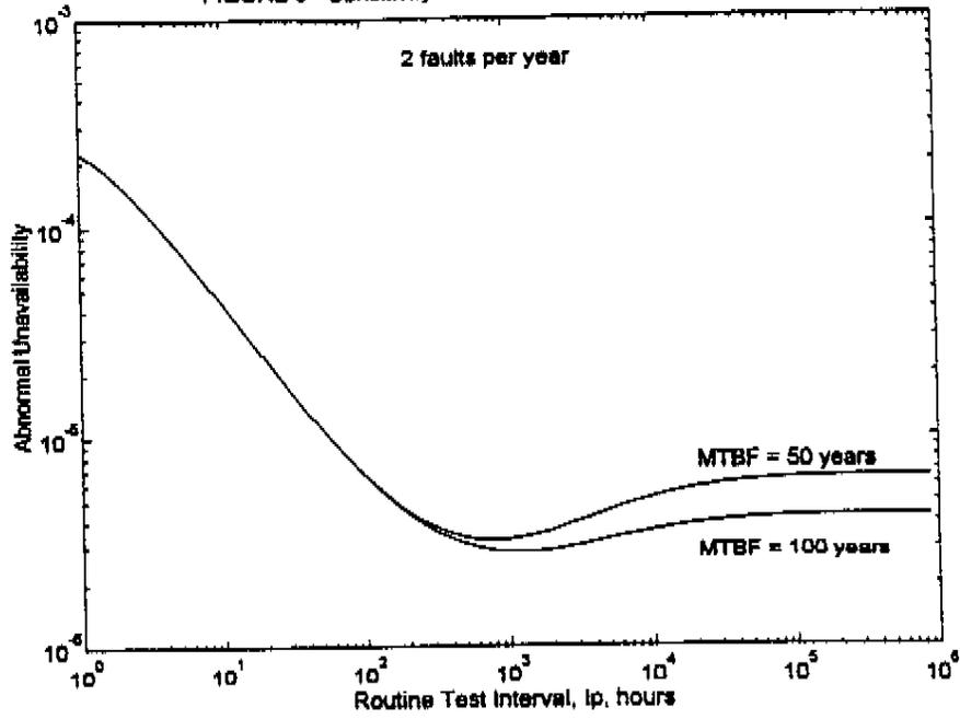
FIGURE 4 - Effect of Self-Tests on Protection Unavailability
