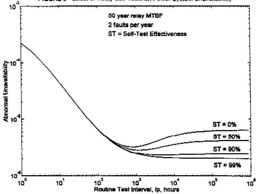
FIGURE 6 - Sensitivity to Faults per Year, Relay With Self-Tests
