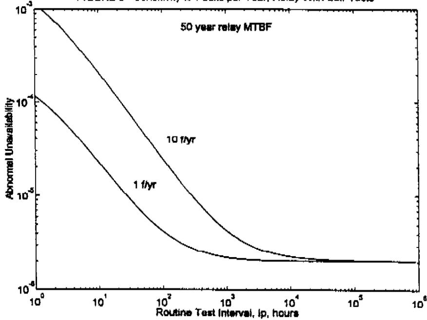
FIGURE 7 - Sensitivity to MTBF, Relay With Self-Tests
