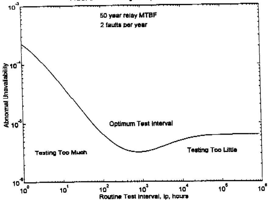
FIGURE 2 - Sensitivity to Faults/Year, Relay Without Self-Tests
