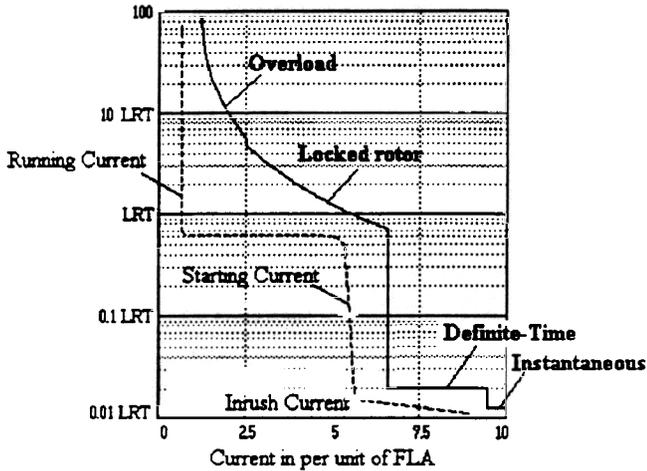
Figure 3: Motor Characteristics Plotted with Motor Starting Current
