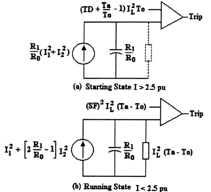
Figure 5: States of the Thermal Model
