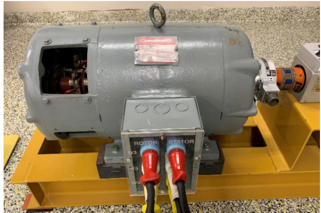
Fig. 7. The 220 V, 10 hp wound-rotor asynchronous machine used for verifying the 87SR element principle of operation.
