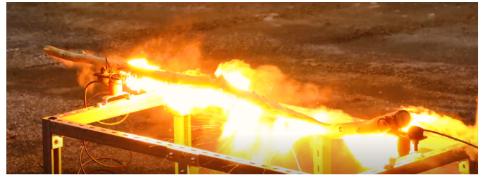
Fig. 8. Last test at Location 2 with 0 ohms added series resistance. Final stages of the fault involved a violent explosion around the faulted branch.
