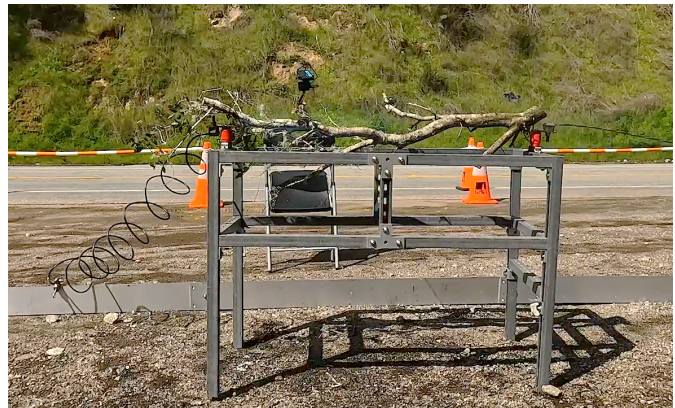
Fig. 3. Wire-on-tree-branch apparatus at Location 2.
