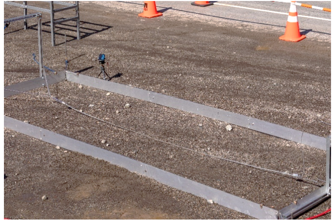
Fig. 2. Wire-on-ground apparatus at Location 2.
