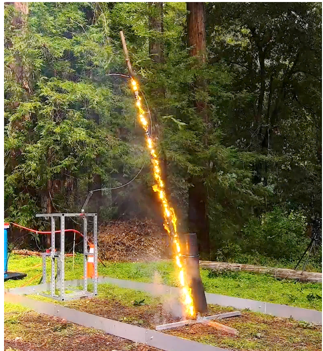
Fig. 13. Location 3: Image of the long redwood branch on fire due to multiple arcs forming on the surface.
