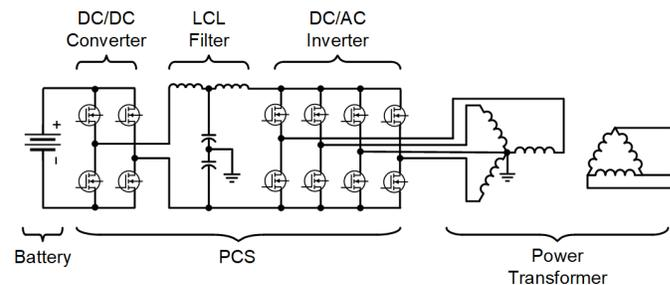
Fig. 6. Four-wire, MOSFET, single-level, two-stage inverter
