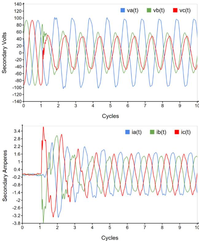
Fig. 35. Transmission-connected GFM IBR transmission substation voltage and current response to nearby distribution fault
