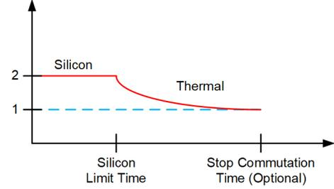
Fig. 9. Inverter current limits
