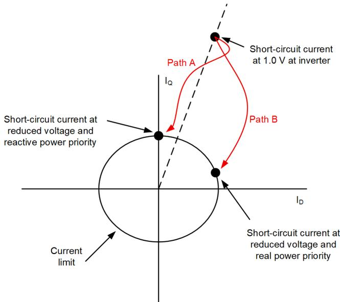
Fig. 14. Faulted circuits require inverters to pull back
