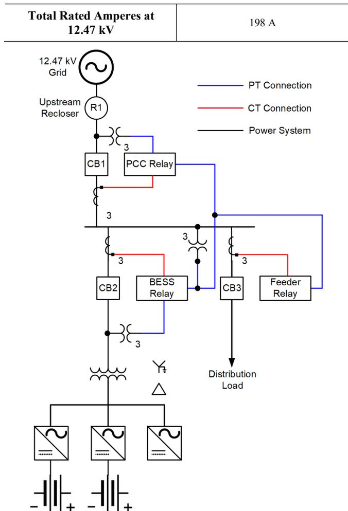
Fig. 21. Distribution system example
