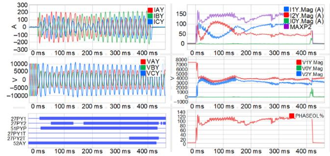
Fig. 30. ER 8 upstream LL distribution fault
