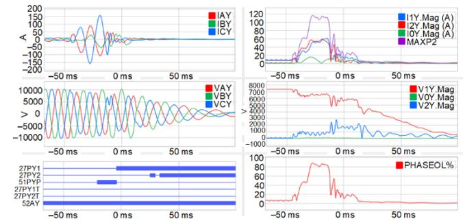
Fig. 24. ER 3 upstream LL transmission fault
