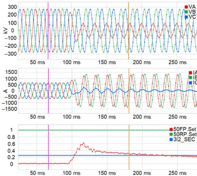
Fig. 42. Relay observations at Bus 10
