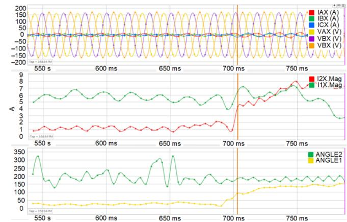
Fig. 37. Removing Phase C with inverter in GFM mode and paralleled to generator
