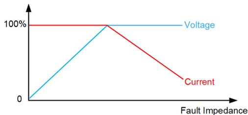
Fig. 10. Fault impedance means different demands on battery
