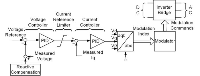
Fig. 8. Reactive power and voltage control
