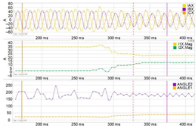
Fig. 13. GFM inverter carrying unbalanced load on island
