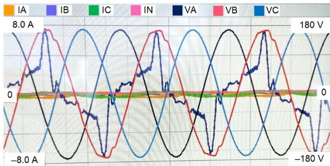
Fig. 17. 1 MHz capture of GFM inverter operating on an island
