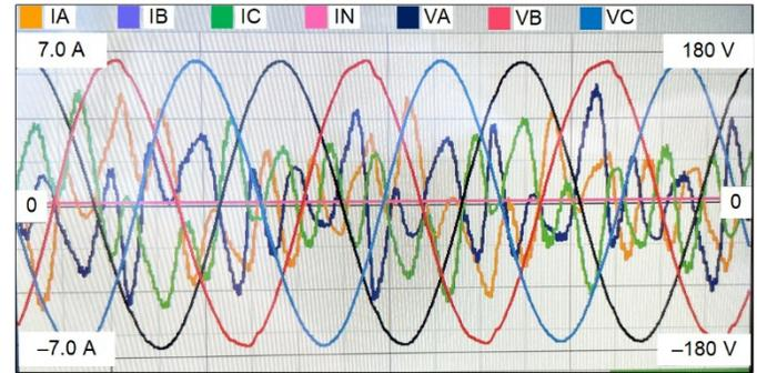
Fig. 18. 1 MHz capture of GFM inverter operating parallel to a generator
