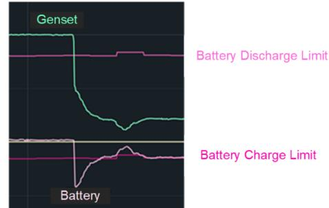
Fig. 3. Lead battery pushed past charge limit to support ac grid
