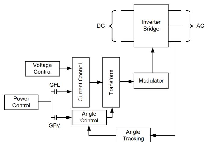
Fig. 4. A typical inverter control system
