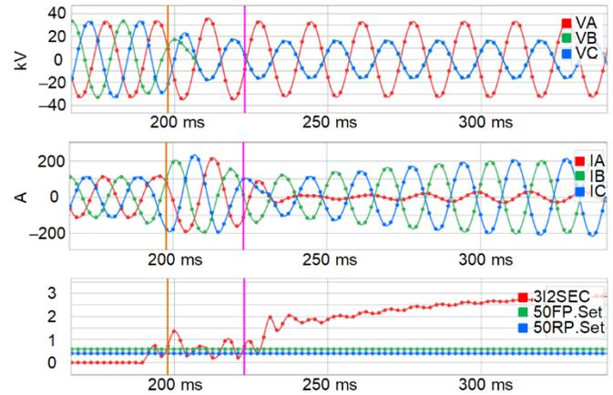
Fig. 40. 50 percent Phase B to Phase C fault measured by R1
