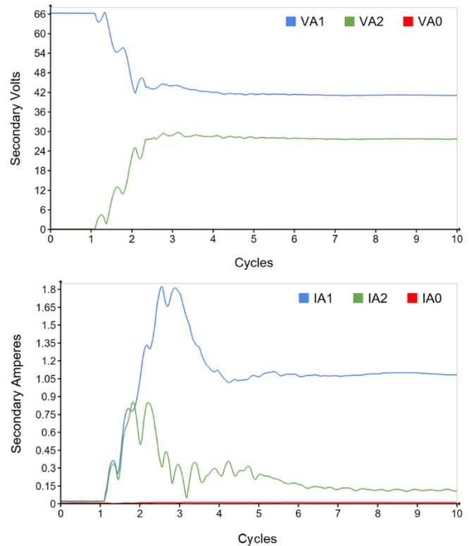
Fig. 36. Sequence voltages and currents for transmission-connected GFM IBR transmission substation voltage and current response to nearby distribution fault
