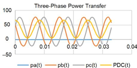
Fig. 11. I2 creates 120 Hz ripple on dc bus
