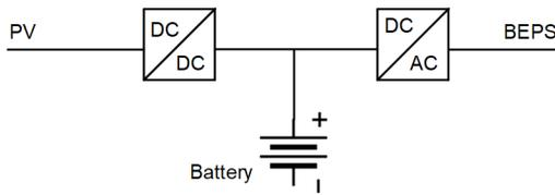
Fig. 34. BESS with dc-coupled PV facility
