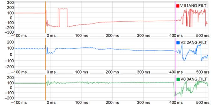
Fig. 31. ER 8 upstream LL distribution fault – V and I angle
