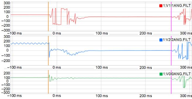
Fig. 27. ER 5 upstream LLG distribution fault – V and I angle
