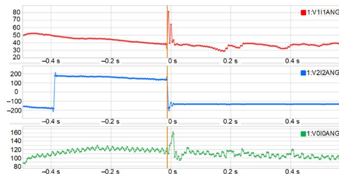
Fig. 23. ER 1 downstream LL distribution fault – V and I angle
