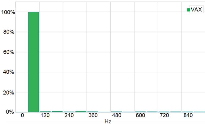
Fig. 16. Relay could not detect the generator slot harmonics
