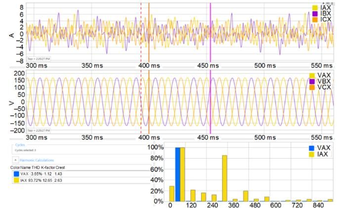
Fig. 19. Relay detected strong fifth- and seventh-harmonic currents but a clean voltage waveform
