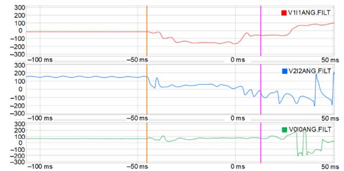
Fig. 25. ER 3 upstream LL distribution fault – V and I angle
