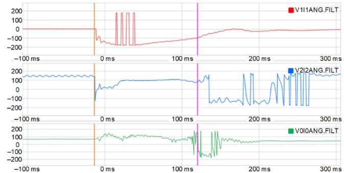
Fig. 33. ER 10 upstream LL distribution fault – V and I angle
