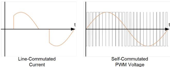
Fig. 2. Comparison of IBR commutation methods
