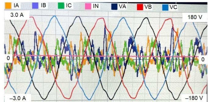
Fig. 20. 1 MHz capture of GFL inverter operating parallel to a generator
