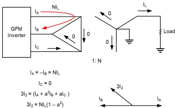
Fig. 12. Calculating natural GFM inverter I2 production
