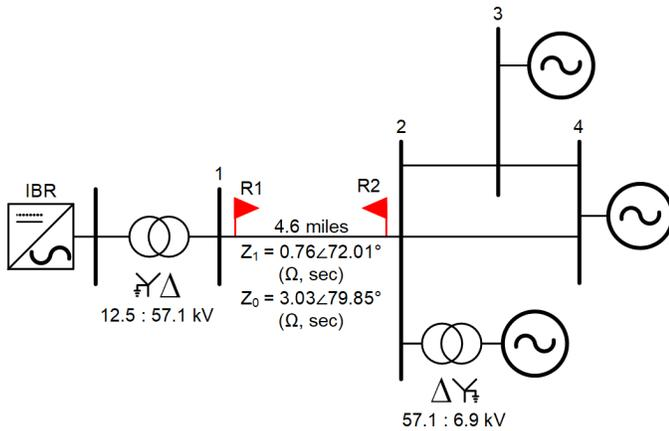
Fig. 39. PV-BESS reduced system
