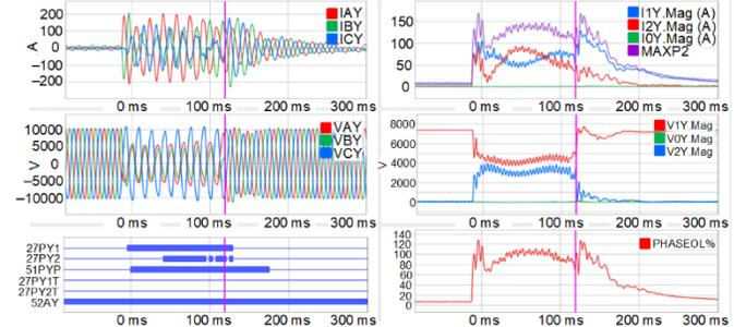
Fig. 32. ER 10 upstream LL distribution fault
