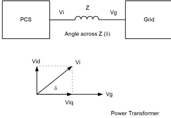
Fig. 7. GFL inverter control of power
