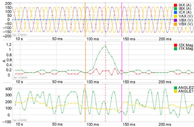
Fig. 38. Removing Phase C with inverter in GFL mode and paralleled to generator
