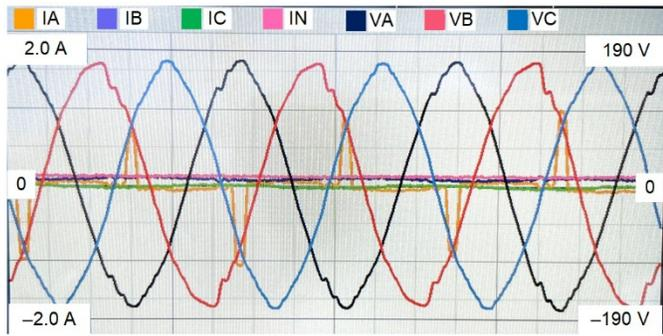
Fig. 15. 1 MHz capture shows generator slot harmonics
