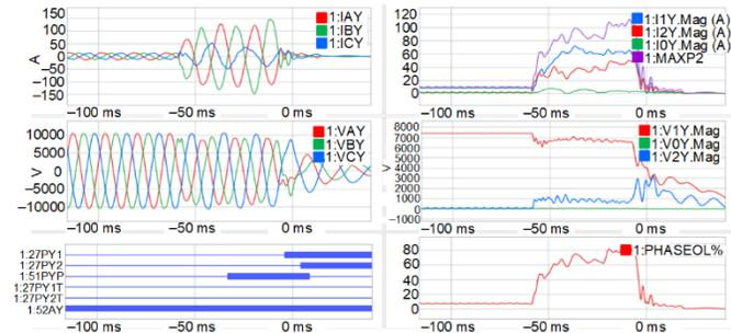
Fig. 22. ER 1 downstream LL distribution fault
