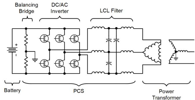
Fig. 5. Three-wire, IGBT, single-level, single-stage inverter
