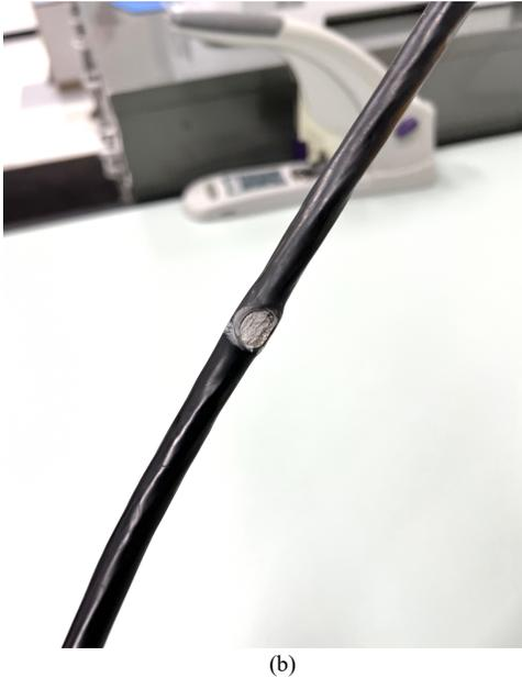
Fig. 7 (a) Service point outside the vineyard; (b) insulation leak found
