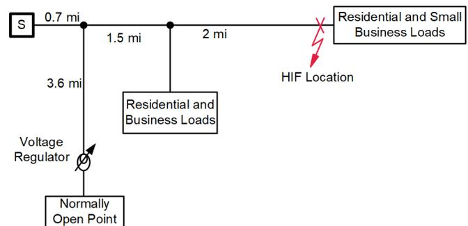
Fig. 1 One-line diagram shows the location of the loose jumper
