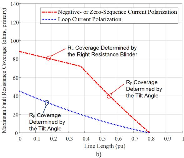
Fig. 14. Maximum fault resistance coverage using negative-sequence-, zero-sequence-, and loop current-polarized reactance elements for a) outgoing load ( $\delta = -10^\circ$ ) and b) incoming load ( $\delta = 10^\circ$ ).
