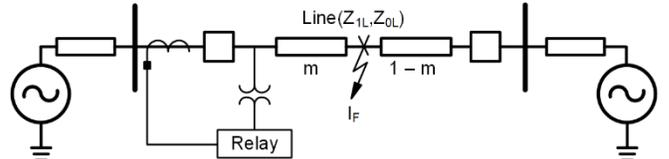
Fig. 3. Two-source power system with a single-line-to-ground fault at a distance  $m$  (pu) from the relay.
