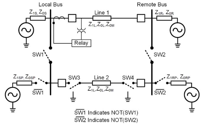
Fig. 15. Network representing various parallel line configurations.
