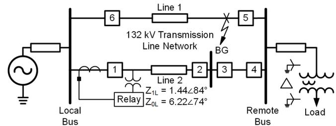
Fig. 24. 10.3 km transmission line (Line 2) connecting two systems with a BG fault on the parallel line (Line 1).
