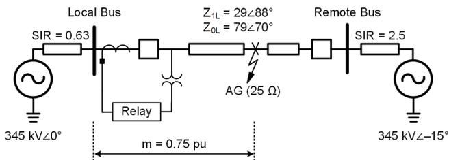
Fig. 10. 50-mile transmission line connecting two systems with an AG fault ( $R_F = 25 \Omega$  primary) at  $0.75$  pu from the local terminal.
