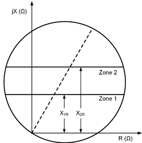
Fig. 1. Operating characteristics of the initial reactance relay [1].
