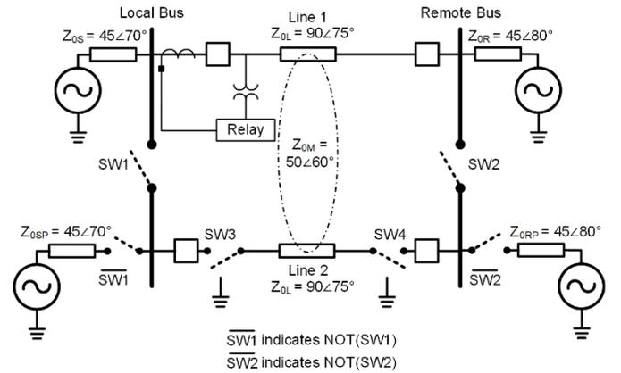
Fig. 29. Network representing various parallel line configurations.
