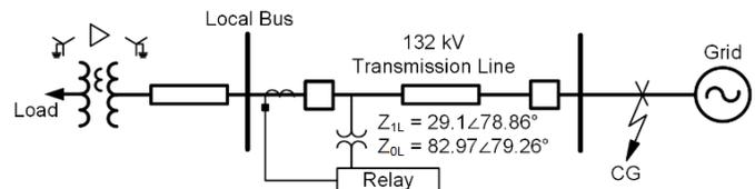
Fig. 20. 87.9 km transmission line with an external CG fault beyond the remote terminal.
