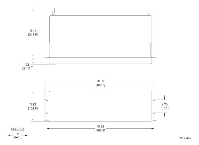
Figure 14 SEL-9L Rack-Mount Dimensions (All Models)
