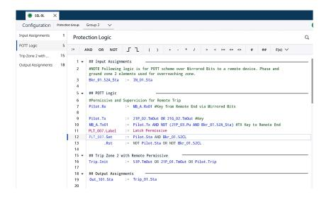
Figure 4 SELogic Editor in Grid Configurator
