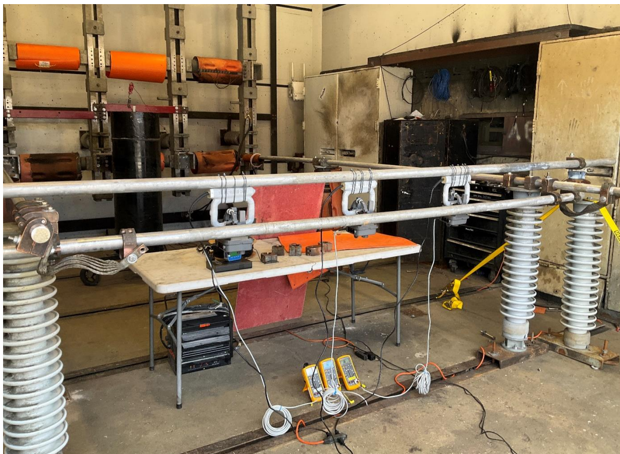
Figure C-5: Test setup for effect of current from adjacent conductor tests.
