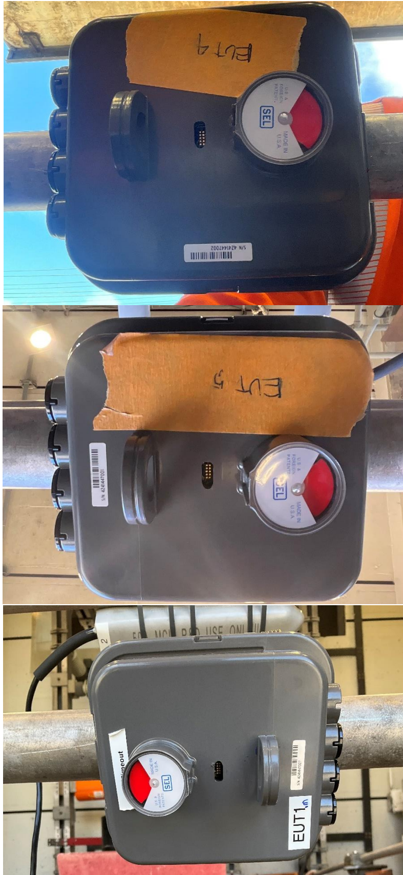
Figure C-9: Samples in trip state after the first 40 kA short-time current test
