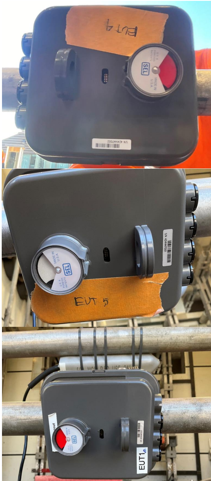
Figure C-10: Sample #5 in normal state after the second 40 kA short-time current test
