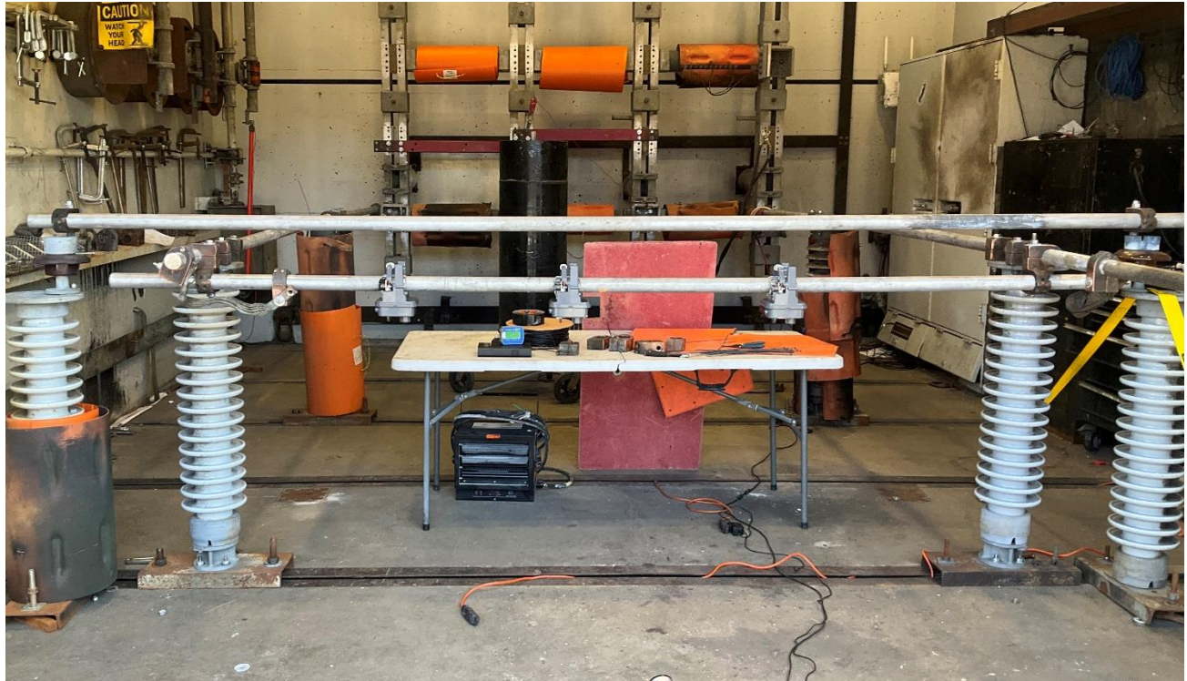
Figure C-6: Test setup for the short-time current tests.
