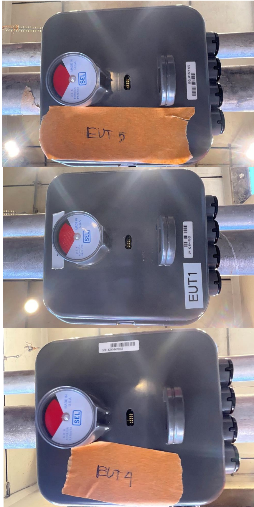
Figure C-8: Samples in trip state after all 25 kA short-time current tests
