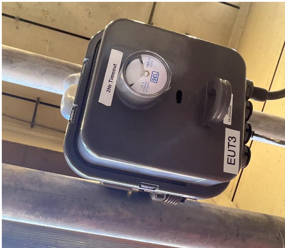
Figure C-7: Sample in normal state after all 25 kA effect of current from adjacent conductor tests
