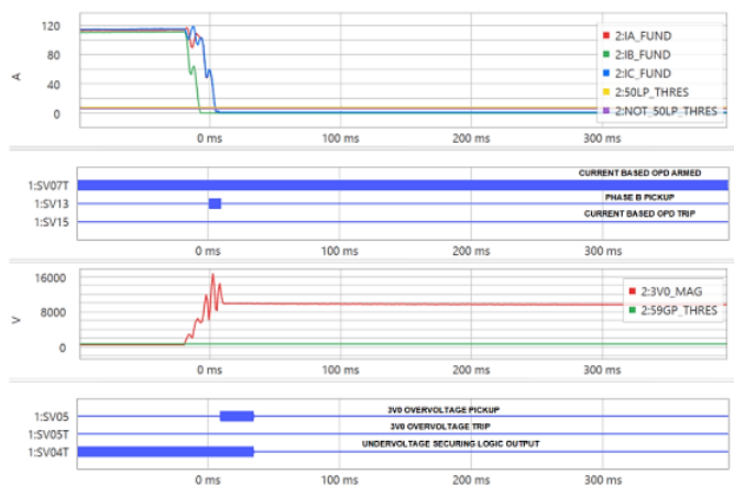
Fig. 16. Open Phase-B Event on a 3-limb Dy11 Transformer Under 90% Loading.
