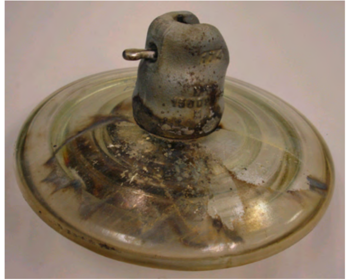
Fig. 1. A flashed insulator bell identified by a patrol crew: UBP of Bonneville Power Administration [3].
