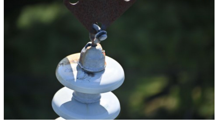
Fig. 8. A flashed insulator identified by the aerial patrol crew.
