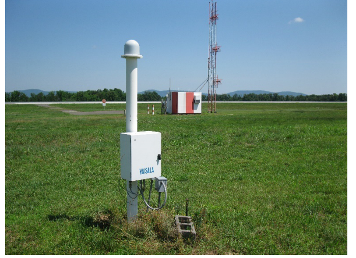
Fig. 5. Lightning sensors measure RF pulses generated by lightning activity.
