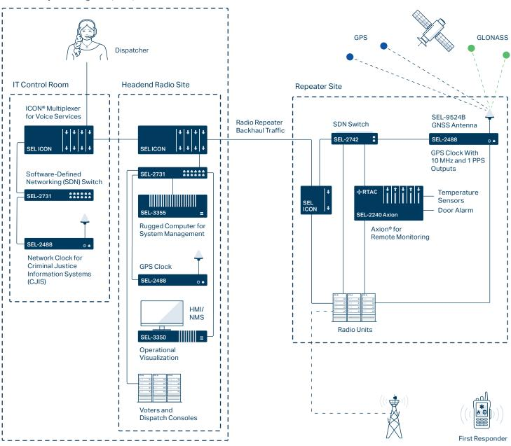
LMR system solutions from SEL incorporate devices that provide precise timing, resilient and cybersafe networking, remote monitoring, and rugged computing.
