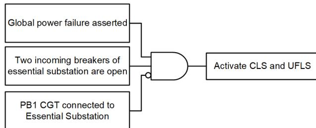
Fig. 6 Logic diagram to activate CLS and UFLS.
