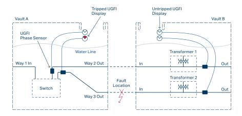
Apply UGFIs to outgoing ways of switches and transformers to determine if the fault is beyond the installed (or monitored) location.
