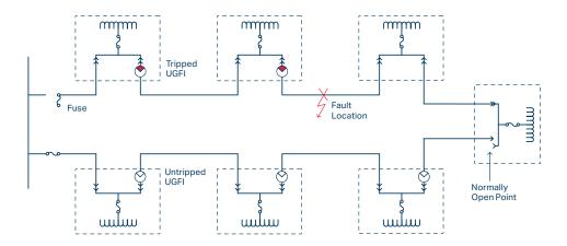
The UGFIs identify the faulted cable section within a loop of pad-mounted transformers that contain a normally open point.
