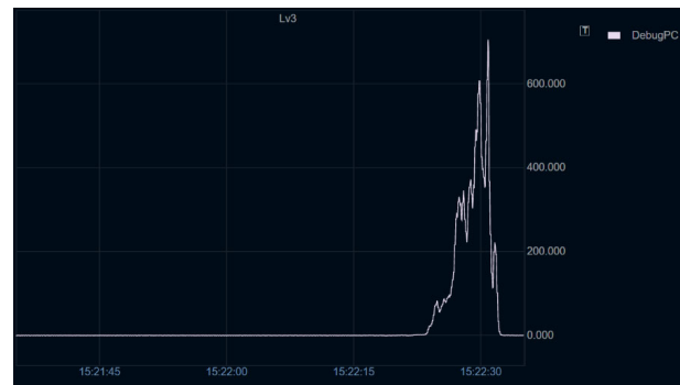
Figure 8 Pyranometer Luminance Sensor Output Displayed in Synchrowave Monitoring
