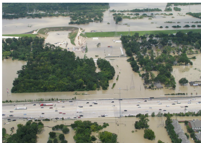
Fig. 9. Addicks Dam cofferdam in February 2018, which was not overtopped and prevented failure of the dam while allowing moderate release of floodwater [22].
