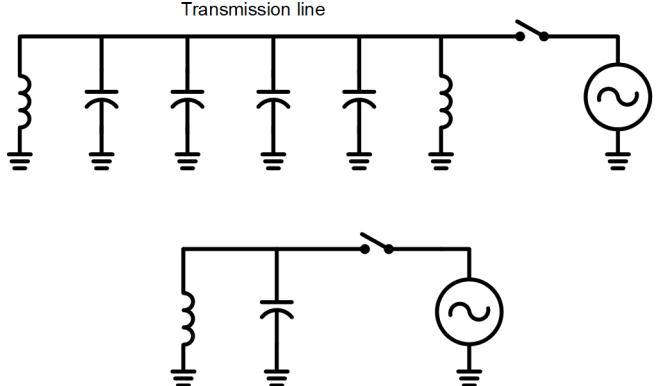
Fig. 5. A shunt-compensated line and its lumped representation.
