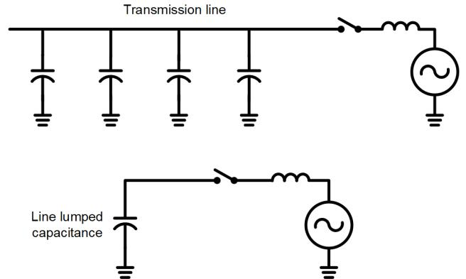
Fig. 1. EHV line with an inherently distributed capacitor and its lumped representation.
