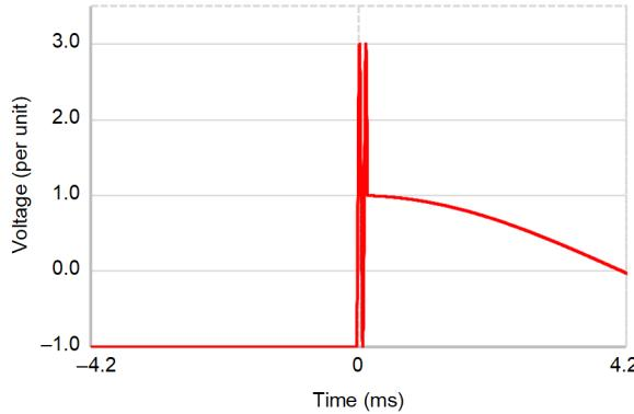
Fig. 2. Switching transients approaching 3 pu in the capacitive network.
