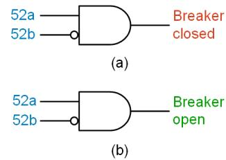
Fig. 22. Use of both breaker 52a and 52b contact inputs for the secure indication of a) the breaker opening and b) the breaker closing.
