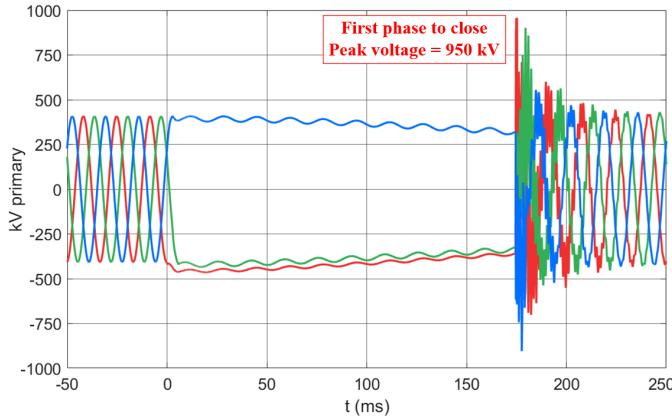
Fig. 3. Switching surges during autoreclose of an uncompensated 500 kV line.
