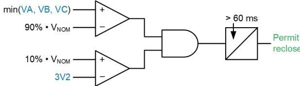
Fig. 24. Follow terminal reclosing supervision using the voltage and a coordination time delay.
