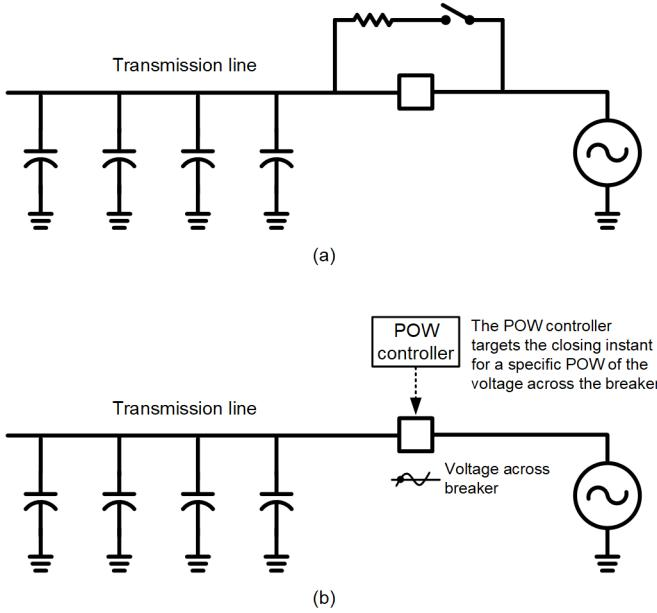
Fig. 4. Control of switching transients in an EHV line using (a) a pre-insertion resistor and (b) POW-controlled closing.
