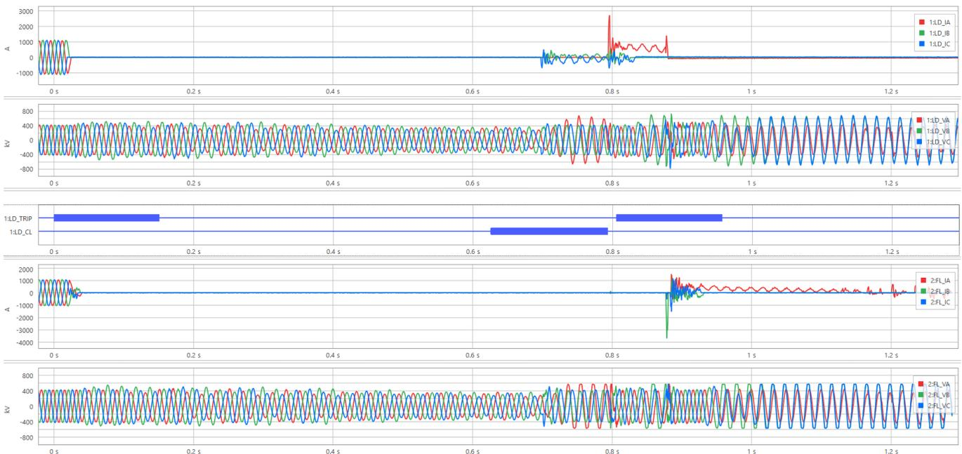
Fig. 13. Protective relay records showing the Event B sequence in the lead and follow terminals. (Note: the follow terminal digitals are not available.)
