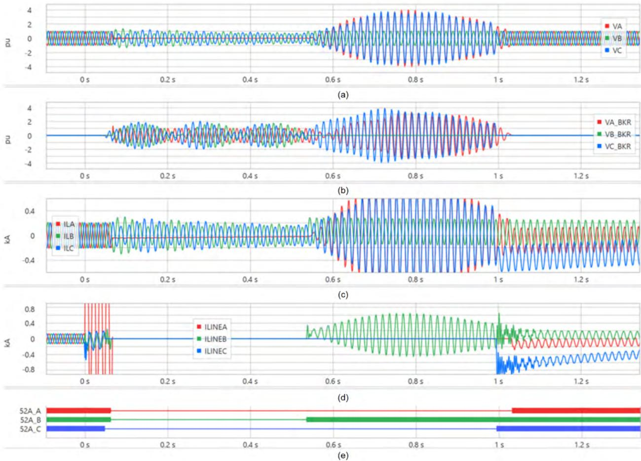
Fig. 8. Missing current zero-crossings, significant overvoltages, and complex beat patterns in a simulated 80 percent shunt-compensated EHV line. Analog traces from top to bottom: (a) line voltages, (b) voltages across the breaker, (c) inductor currents, and (d) line currents.
