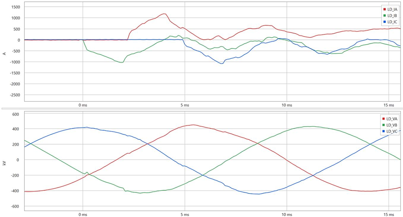
Fig. 11. Three-phase line currents and voltages at the lead terminal during manual energization via POW on May 14, 2021.
