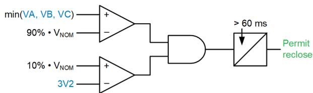
Fig. 24. Follow terminal reclosing supervision using the voltage and a coordination time delay.
