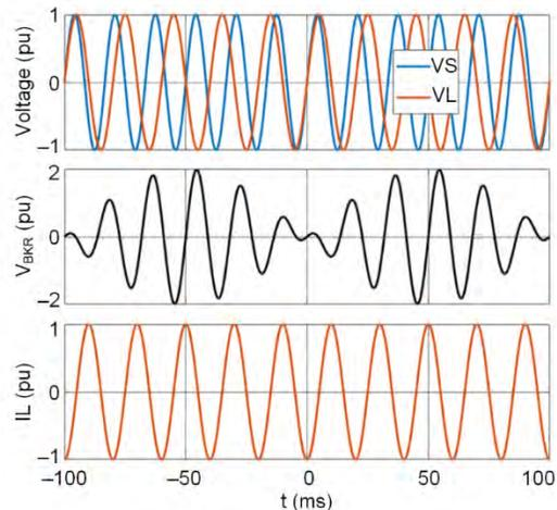
Fig. 7. The source voltage ( $V_S$ ), line ringdown voltage ( $V_L$ ), voltage across the closing breaker ( $V_{\text{BKR}}$ ), and reactor current ( $I_L$ ) during a three-phase open time interval.
