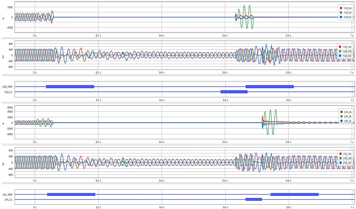
Fig. 19. Protective relay records showing the Event E sequence in the lead and follow terminals.
