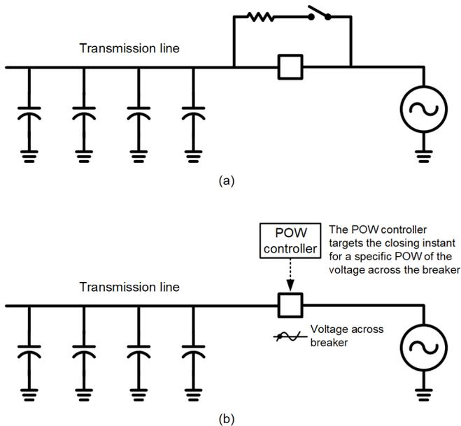
Fig. 4. Control of switching transients in an EHV line using (a) a pre-insertion resistor and (b) POW-controlled closing.
