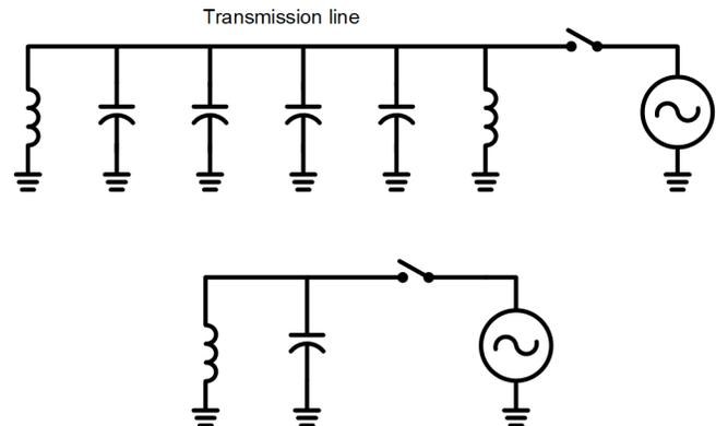
Fig. 5. A shunt-compensated line and its lumped representation.
