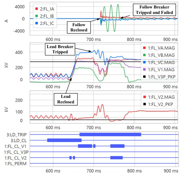
Fig. 25. Secure performance of reclose supervision logic for Event E. Analog traces from top to bottom: (1) follower breaker three-phase current, (2) follower breaker line voltage measurements and threshold, and (3) follower breaker line negative-sequence voltage and threshold.
