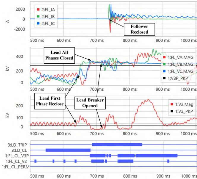
Fig. 26. Secure performance of reclose supervision logic for Event C. Analog traces from top to bottom: (1) follower breaker three-phase current, (2) follower breaker line voltage measurements and threshold, and (3) follower breaker line negative-sequence voltage measurement and threshold.
