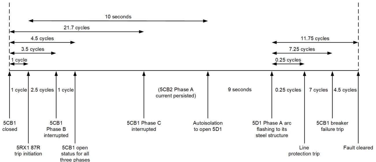
Fig. 10. Detailed sequence of events during the failure of the 5CB1 breaker at the lead terminal on May 14, 2021.
