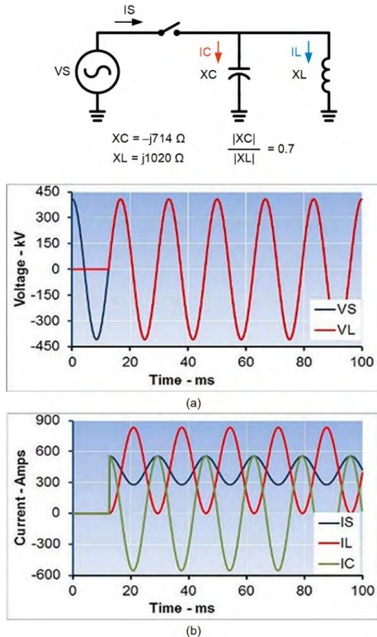
Fig. 6. Switching (a) voltage and (b) current in a 70 percent compensated line with target closing at voltage zero across the breaker.
