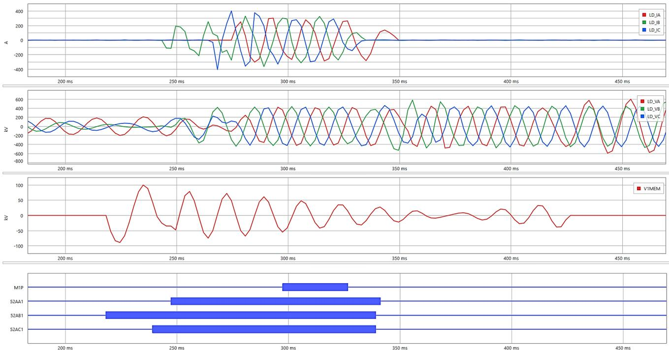
Fig. 21. The relay event record at the lead terminal showing memory charging upon closing of the auxiliary contact but before closing of the main power contacts on July 12, 2016.
