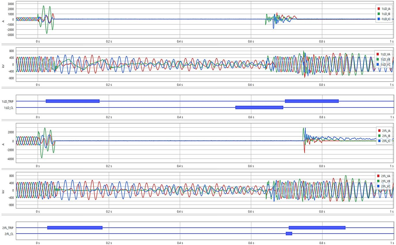
Fig. 15. Protective relay records showing the Event C sequence in the lead and follow terminals.
