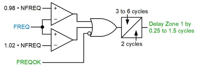
Fig. 28. Zone 1 delay using frequency supervision.
