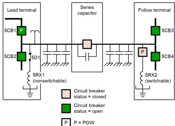
Fig. 9 Generic one-line diagram of the 500 kV lines involved in failure events. The series capacitor was bypassed and not relevant.
