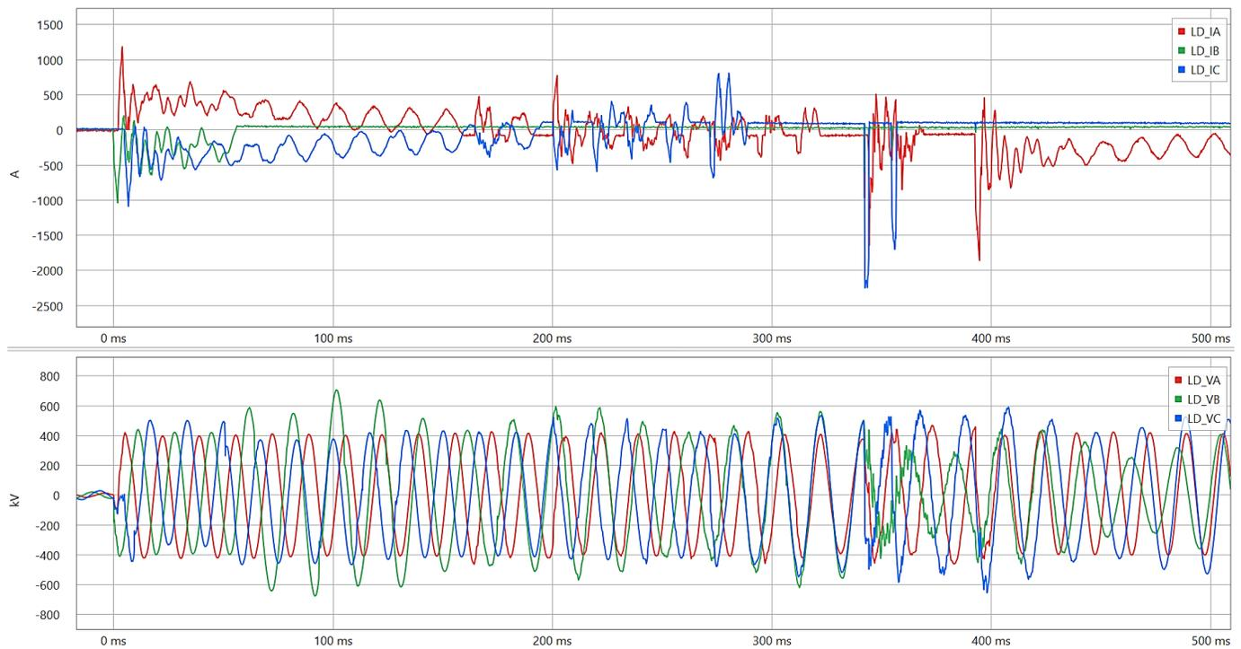
Fig. 12. The first 30 cycles of 5CB1 currents and terminal voltages after breaker closing on May 14, 2021.
