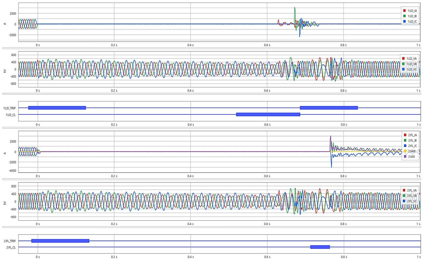
Fig. 17. Protective relay records showing the Event D sequence in the lead and follow terminals.
