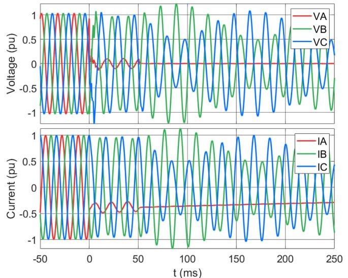
Fig. 23. Missing zero-crossings in the reactor current after a line Phase A-to-ground fault.
