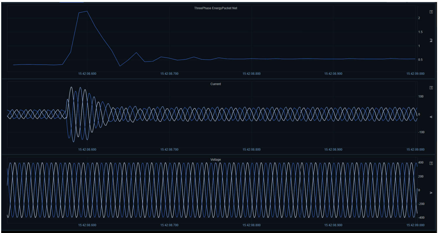
Visualize the energy required to start a motor.
