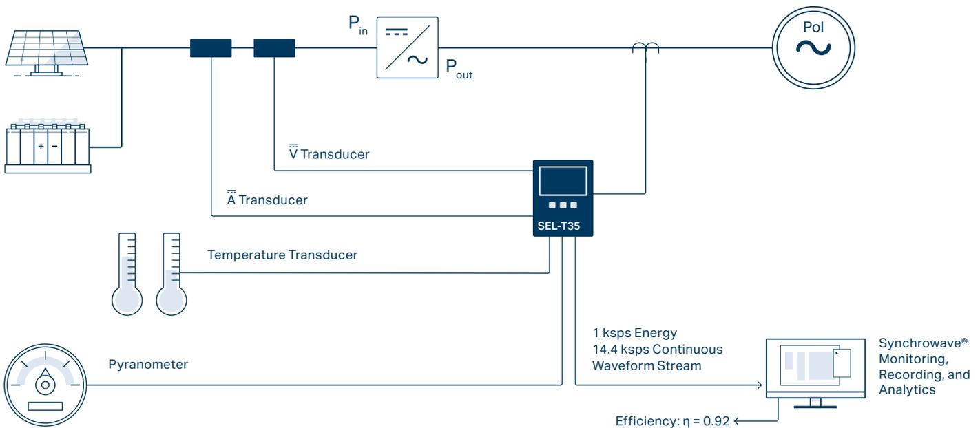
Measure production and calculate power conversion efficiency and distortion.
