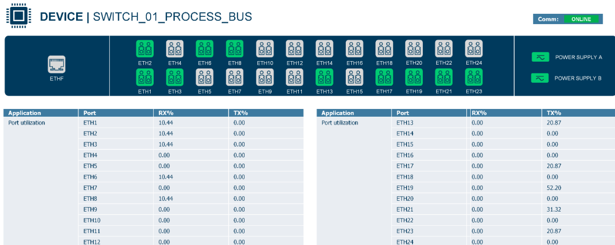
Fig. 15. Ethernet switch monitoring screen.
