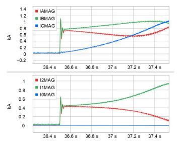
Fig. 8. Phase and sequence currents of a bolted AB fault when the inverter is in Droop mode
