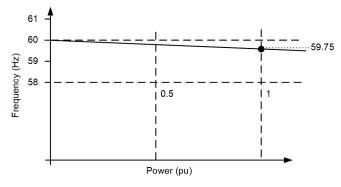
Fig. 7. Droop control characteristics
