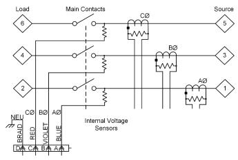
Fig. 12. Recloser controller secondary voltage connections
