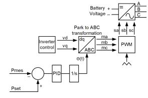
Fig. 6. GFM inverter control [3]
