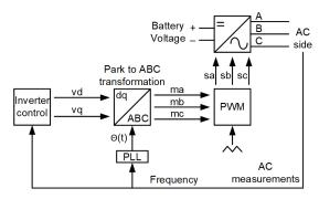
Fig. 5. GFL inverter control [3]
