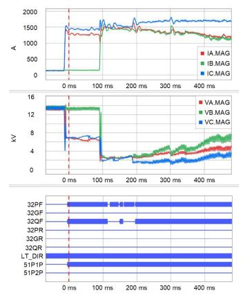
Fig. 10. Evolving fault at RCL6
