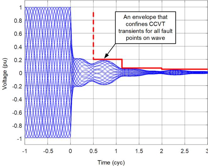
Fig. 5. Transient envelope for all possible CCVT transients for a given CCVT make and model.
