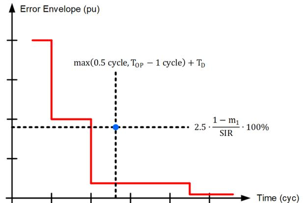
Fig. 9. Graphical illustration of the CCVT transient security condition.
