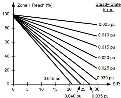
Fig. 14. Zone 1 security chart considering steady-state errors.
