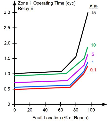
Fig. 11. Zone 1 operating time curves (Relay B).
