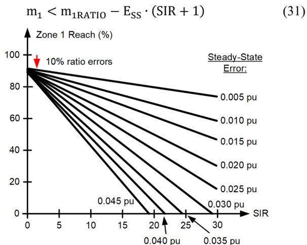
Fig. 19. Example Zone 1 security chart considering 10 percent ratio error and a range of fixed steady-state errors.
