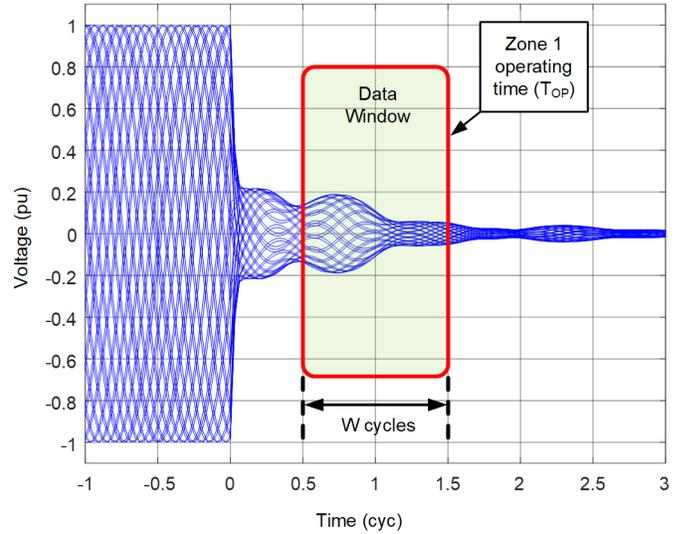
Fig. 4. Sample CCVT transient and the relay data window at the time of Zone 1 operation.
