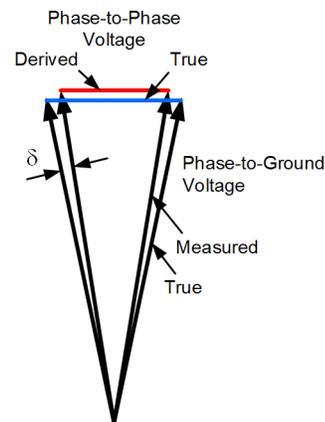
Fig. 16. Illustration of the measuring error in phase-to-phase voltage derived from two phase-to-ground voltages.
