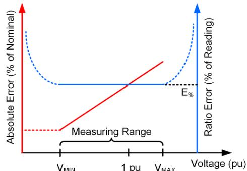
Fig. 15. Measuring range, ratio error (blue), and absolute error (red).
