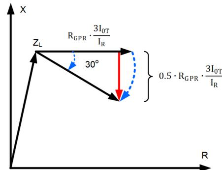
Fig. 18. Impact of the GPR on the distance element apparent impedance in homogeneous and nonhomogeneous networks.
