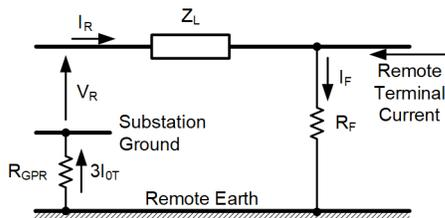
Fig. 17. Impact of the GPR on the ground loop distance measurement.
