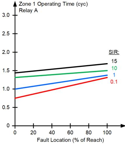
Fig. 10. Zone 1 operating time curves (Relay A).
