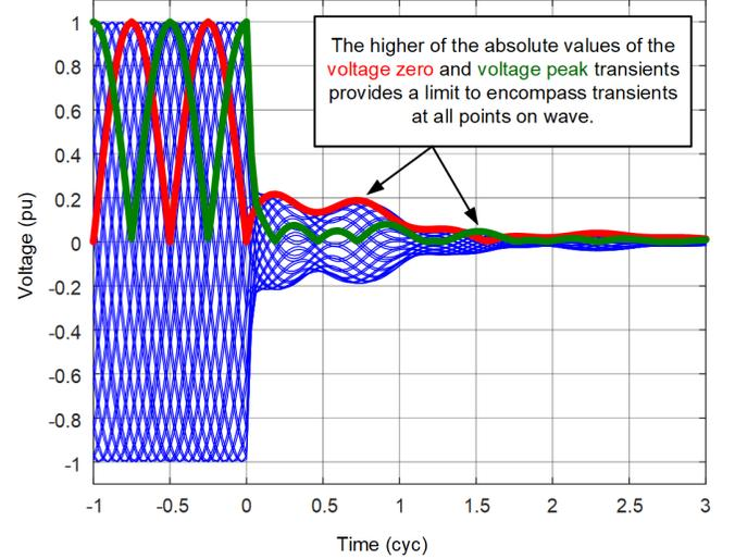
Fig. 7. Obtaining the CCVT transient envelope based on the absolute value of the secondary voltage plots for the fault at voltage zero (red) and voltage peak (green).
