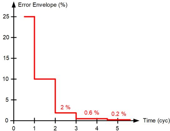
Fig. 6. Sample CCVT transient envelope (Class 3PT2 per IEC 61869-5 [7]).
