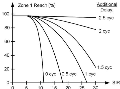
Fig. 13. Proposed Zone 1 security chart (specific to a given CCVT class and relay make and model).
