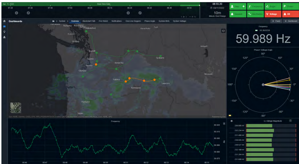
Fig. 1. Example of a synchrophasor’s wide-area monitoring system.
